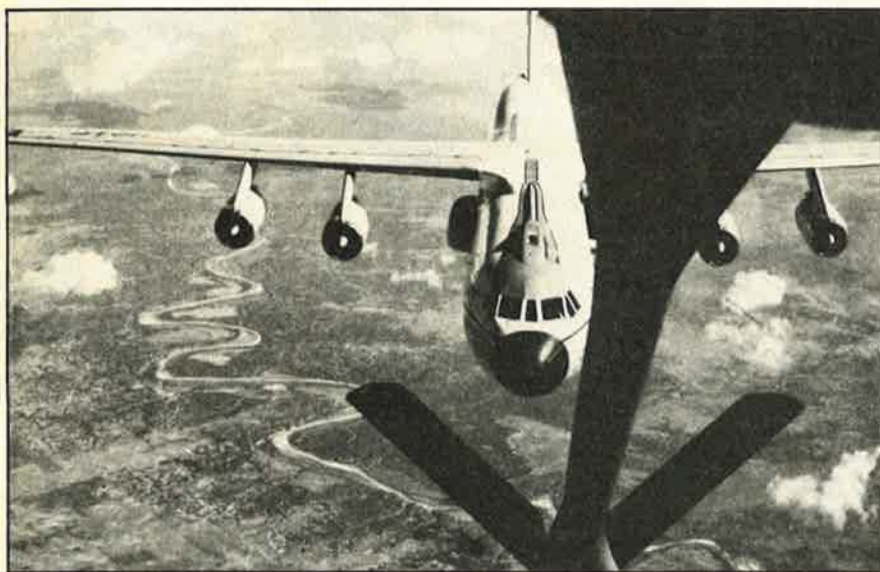
A stretched C-141B StarLifter moves up on a jet tanker refueling boom. Modification of the C-141 fleet to the "B" model should be complete by mid-1982.
