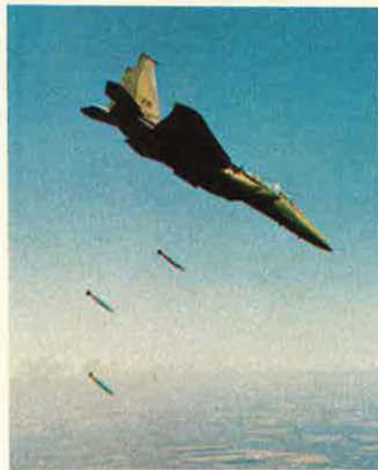
Here, the F-15B delivers two types of ordnance: firing its 30-mm guns, above, and dropping bombs, left. One feature McDonnell Douglas is testing aboard the enhanced Eagle is a maneuvering attack system that will allow bomb drops in attitudes other than wings level.
