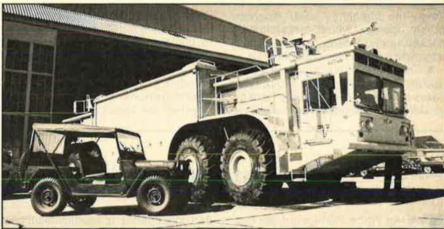
The heavy hitter of the Air Force's fire protection services is the massive and fast two-engine P-15 fire truck.
