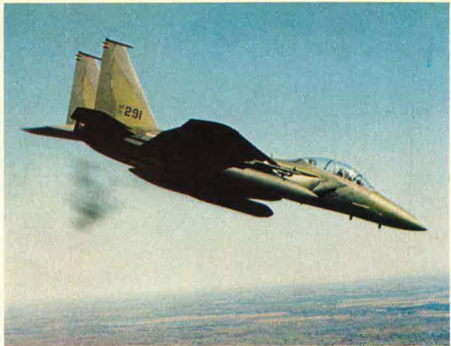
Here, the F-15B delivers two types of ordnance: firing its 30-mm guns, above, and dropping bombs, left. One feature McDonnell Douglas is testing aboard the enhanced Eagle is a maneuvering attack system that will allow bomb drops in attitudes other than wings level.
