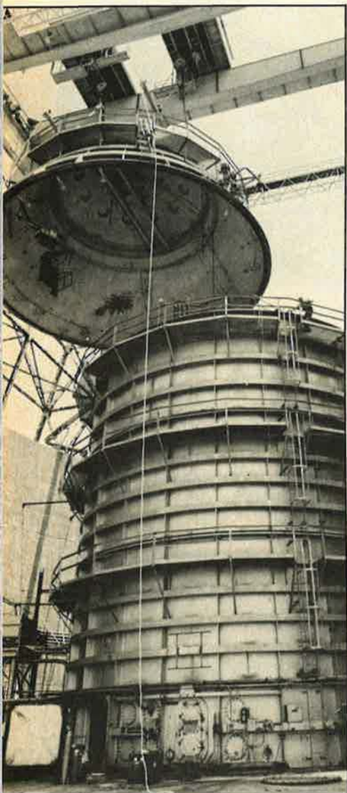
High-altitude rocket test cell—the world's largest—at AFSC's Arnold Engineering Development Center, Arnold AFS, Tenn.
