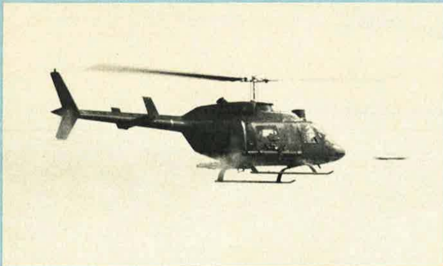
TOW anti-tank missile leaving a TexasRanger during firing trials in the Mojave Desert
