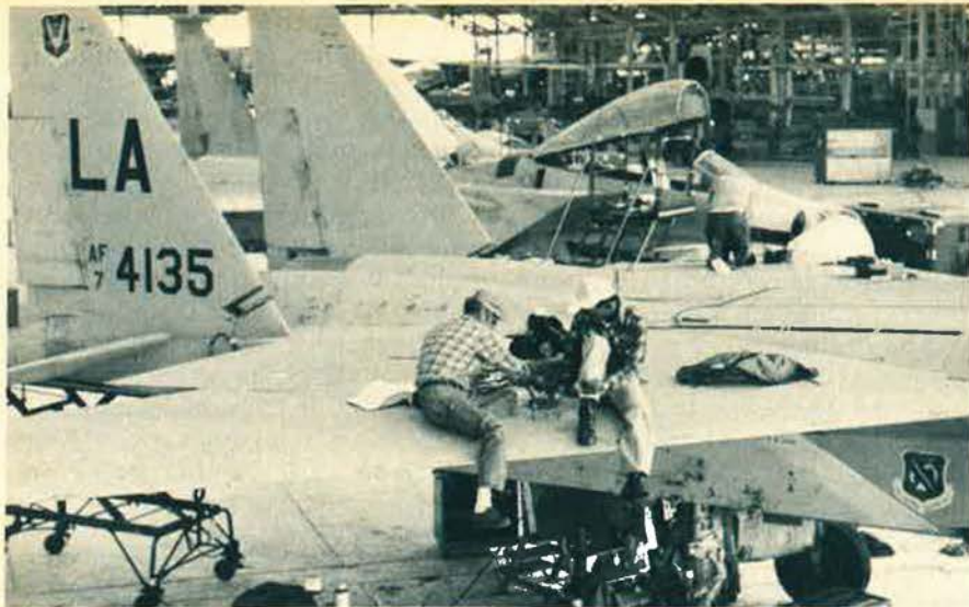
The Warner Robins Speed Line was set up to correct a flaw in the F-15's secondary power system and kept active thereafter in an evolving program of modifications "to enhance performance through state-of-the-art improvements." Here, civilian specialists James Thompson, left, and Wallace Johnson seal a wing fuel tank.
