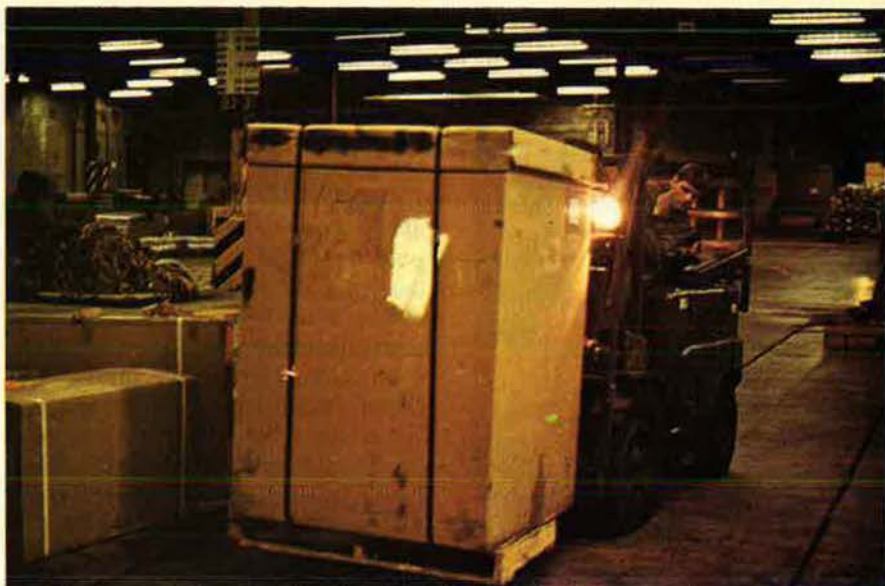
Building up pallets at the 436th Military Airlift Wing's aerial port at Dover AFB, Del. The activity goes on around the clock, building up multiple items into modular-weight (about 3,000 pounds) pallets for onward airlift.
