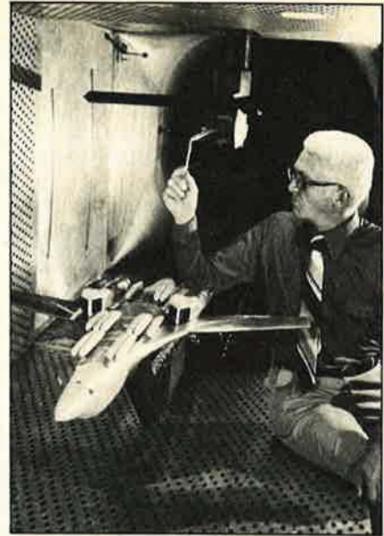
ARO, Inc., engineering supervisor Jack Marshall checks model of Boeing AGM-86B ALCM prior to wind tunnel test aboard model of Rockwell International ALCM launcher aircraft.
