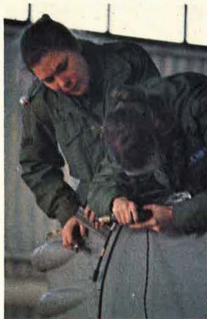
A1C Kimberly Estrada (left) instructs A1C Patricia L. Fischer in the repair of a leading edge crack on the left vertical stabilizer of an F-15 of the 36th Tactical Fighter Wing, Bitburg AB, Germany.
