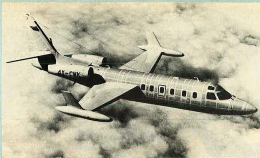
New 'Sigma' wings and winglets identify IAI's Westwind 2, which is produced in parallel with the Westwind 1
