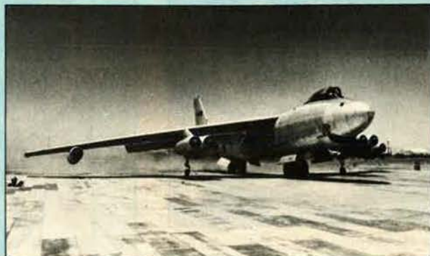
Top photo, Col. George Nakis, left, and Lt. Col. Bob Fawver review B-47 technical data prior to their one-time flight. Above, six jet engines kick up dust as B-47 No. 53-2104 taxis to the flight line.
