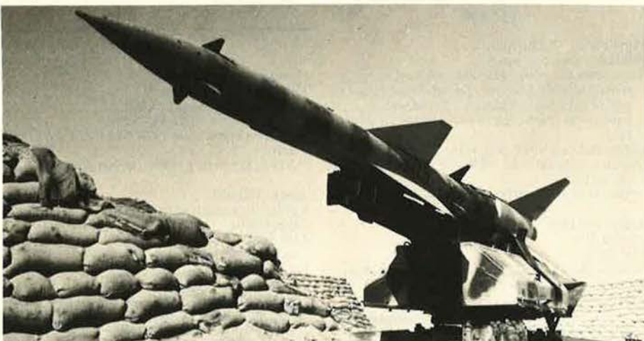
Several countries in the region have these Soviet-built SA-2 SAMs with a slant range of 40 to 50 km, as well as a variety of other Soviet air defence missiles.
