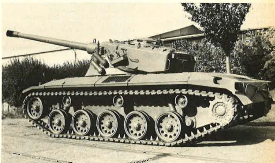
Austria developed and produced this tank destroyer for its army. It has a 105mm antitank gun and is equipped with a laser rangefinder.
