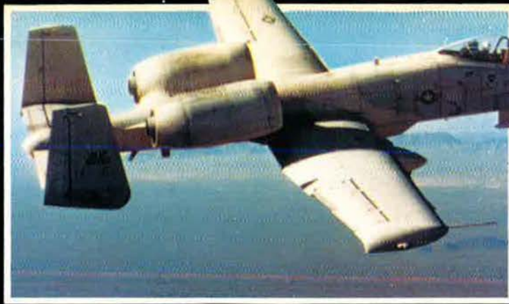
TF34-POWERED A-10 CLOSE AIR SUPPORT AIRCRAFT
