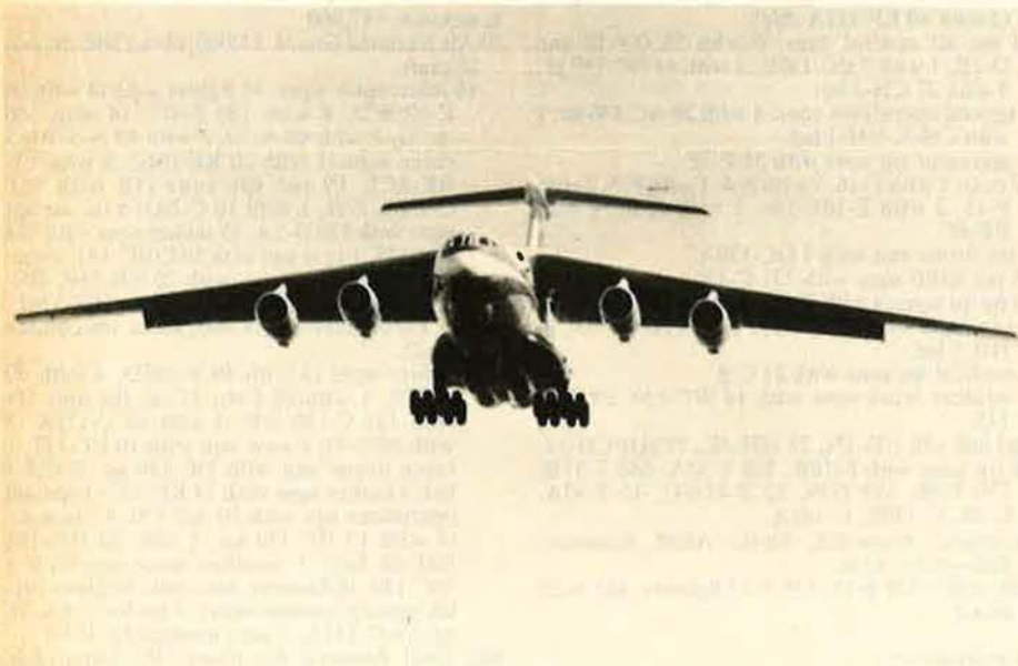
The Il-76 Candid , with a payload of 88,000 pounds, is the USSR's principal long-range transport. It also has been tested as a tanker for the Backfire bomber.
