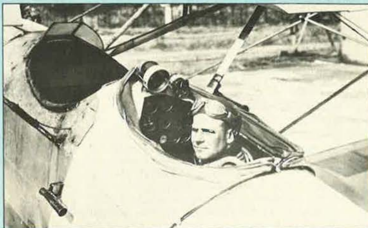
Back then, in 1929, Jimmy Doolittle prepares for the first blind flight, a milestone in aviation progress. Note hood built especially to enclose the cockpit and confine visibility to the instrument panel.
