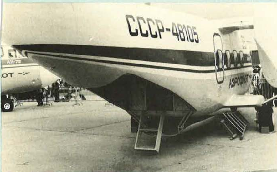
Rear-loading ramp-door of An-28 in forward, underfuselage position
