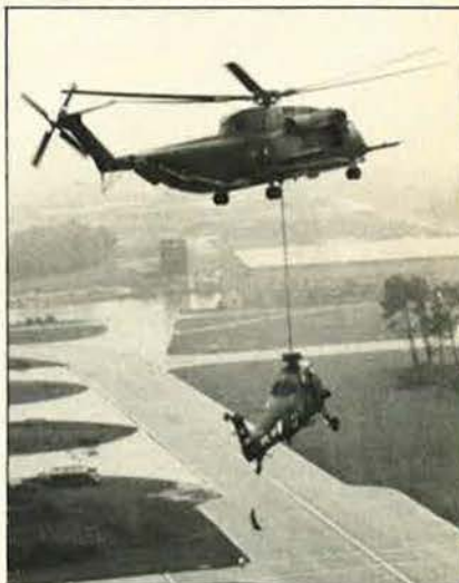
A 67th ARRS HH-53 from RAF Woodbridge, UK, using a special cable designed for Apollo space capsule recoveries, demonstrates airlift capabilities in retrieving a disabled Royal Navy Wessex helicopter.
