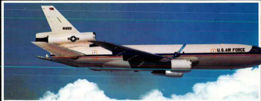
CF6-50-POWERED KC-10A ADVANCED TANKER/CARGO AIRCRAFT
