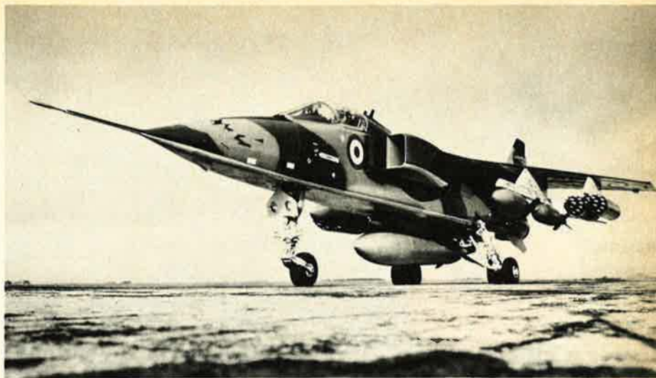
More than 350 British/French Jaguar Mach 1.5 tactical support aircraft have been produced for the RAF and France. Ecuador and Oman also fly the Jaguar.
