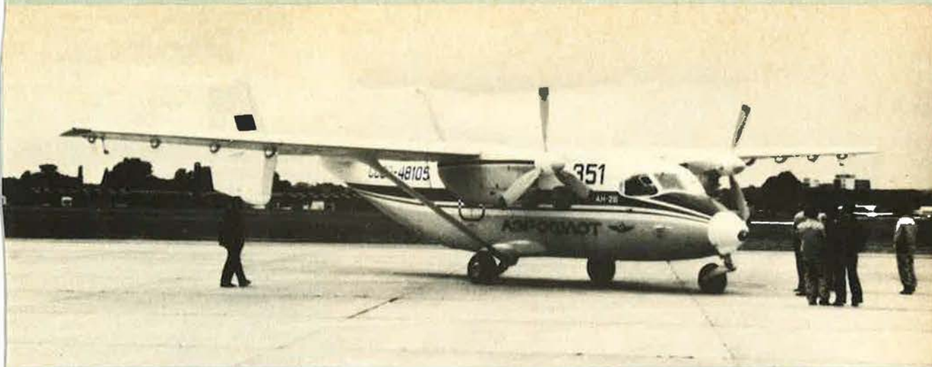
Antonov An-28 light general-purpose transport (two Glushenkov TVD-10B turboprop engines)
