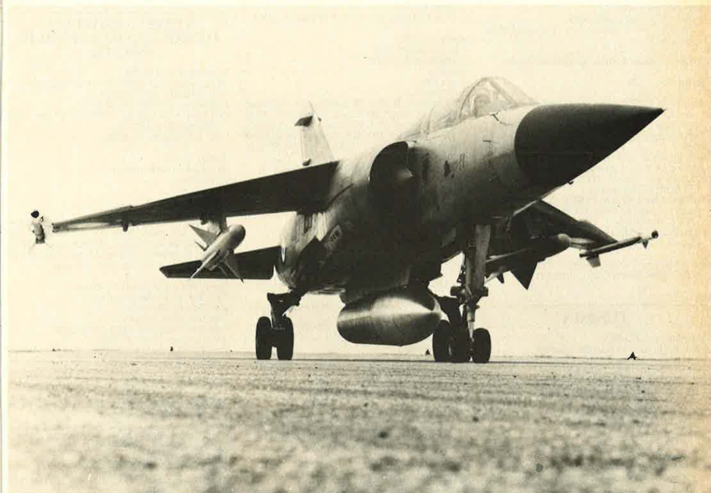
Iraq, Jordan, Kuwait, Libya, and Morocco either have or have on order French Mirage F-1 all-weather interceptors. The F-1, which competed against the US F-16 for selection by four NATO air forces, is a Mach 2.2 aircraft with a ceiling of 65,000 feet.
