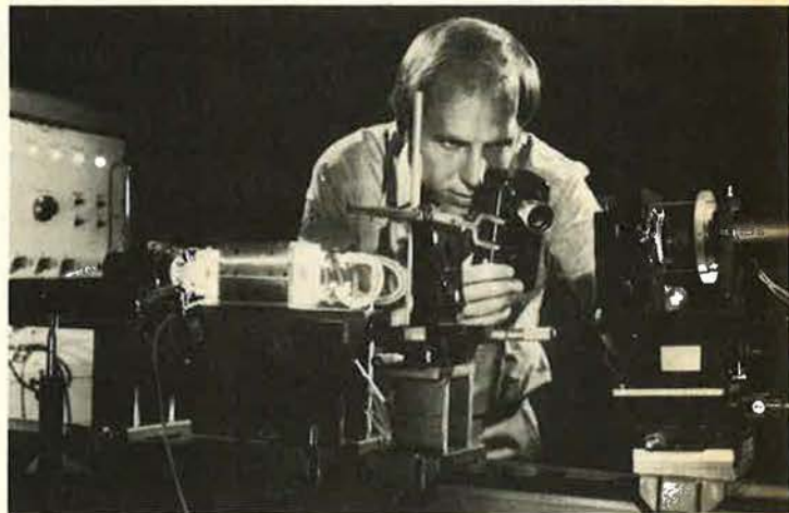
A laser scanner utilizing thermochromic VO 2 .
