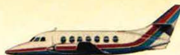
Jetstream 31 – fast, pressurised propjet whose large cabin sets new standards for 19-seat commuter operations.
