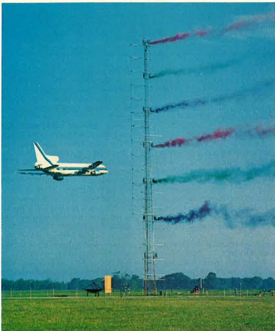
Visual data gathered in a series of wake vortex turbulence tests employing this "smoke tower" was helpful in establishing safe landing separation standards. Wake turbulence had been deemed the culprit in a number of crashes.
