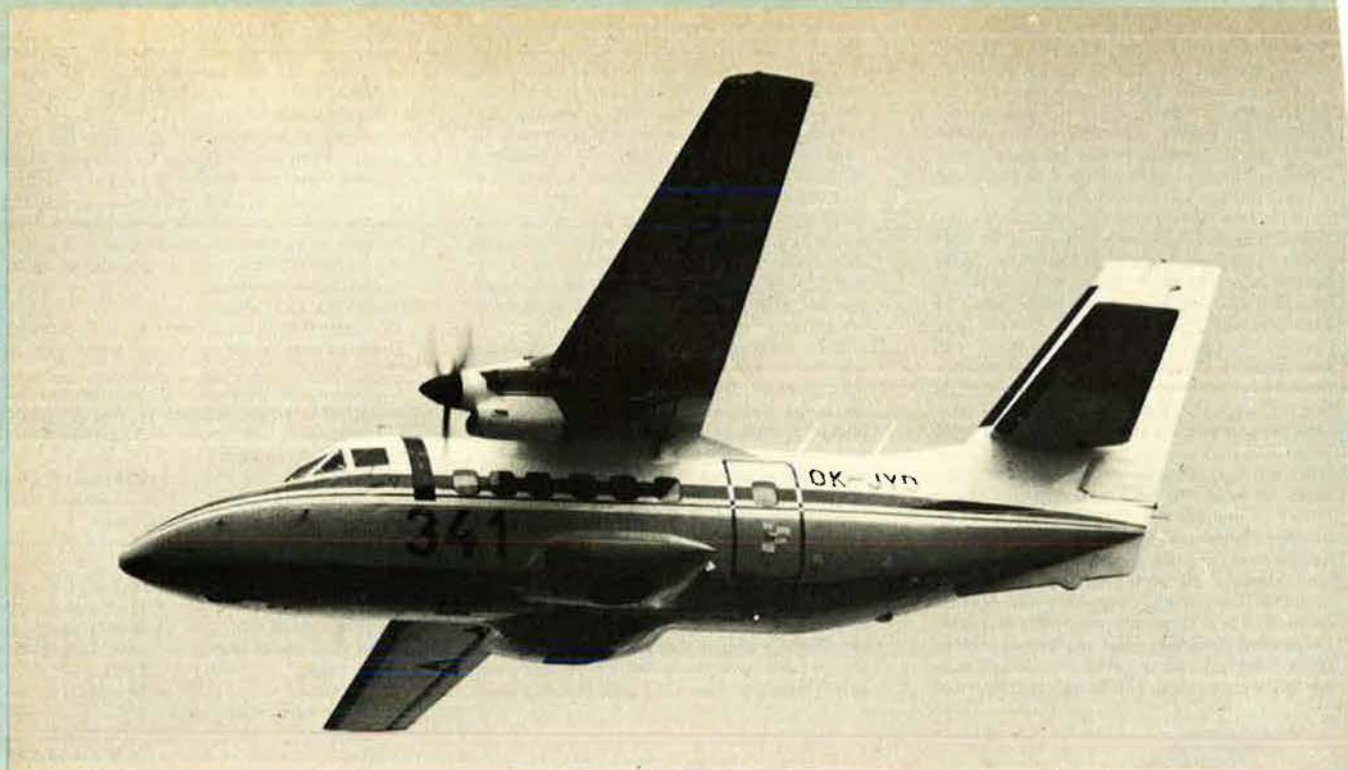
Let L-410UVP twin-turboprop light transport, which is to be built at the rate of about 100 a year for Aeroflot (J.M.G. Gradidge)
