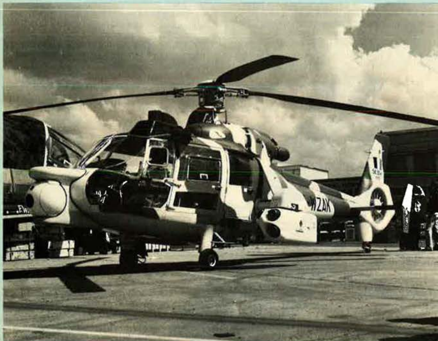
Offered as a light combat helicopter capable of operating on 'starry nights', the Aerospatiale SA 361H/HCL now has its eight Hot anti-tank missiles supplemented by a nose-mounted FLIR (forward looking infra-red) pod ( Brian M. Service )
