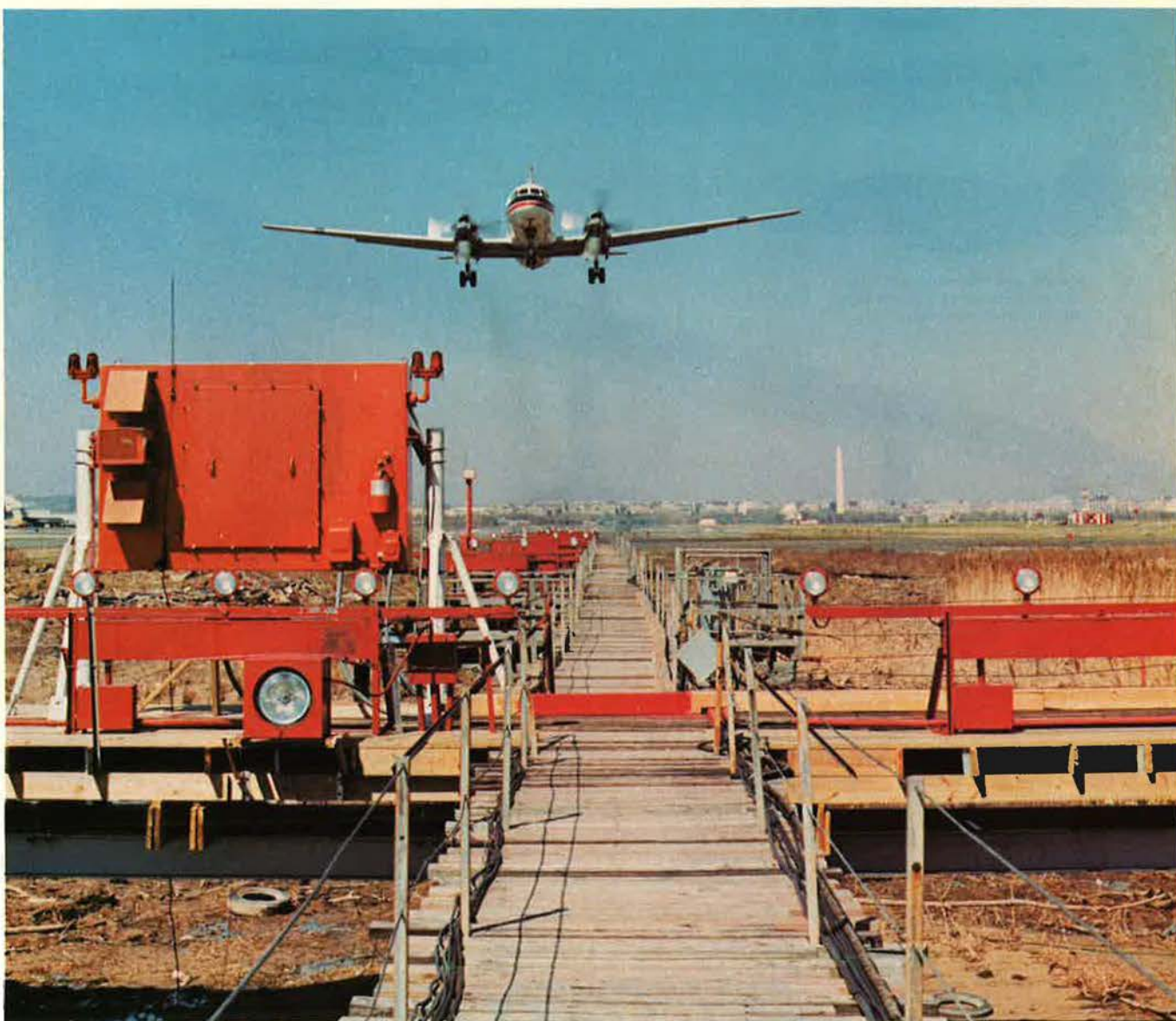
At Washington's National Airport, a NAFEC aircraft checks out effectiveness of the new Microwave Landing System.
