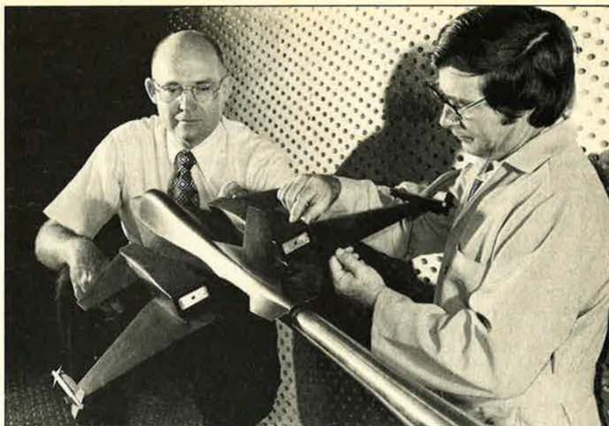
A scale model of a possible fighter of the future featuring vectored engine-over-wing design was recently the subject of wind-tunnel tests at Arnold Engineering Development Center, Arnold AFS, Tenn. The concept is intended to enhance the aircraft's low- and high-speed maneuverability as well as providing for short-field takeoff and landing. Test conditions simulated flights at speeds from Mach 0.2 to 1.97 (150 to 1,400 mph; 240 to 2,250 km/h).
