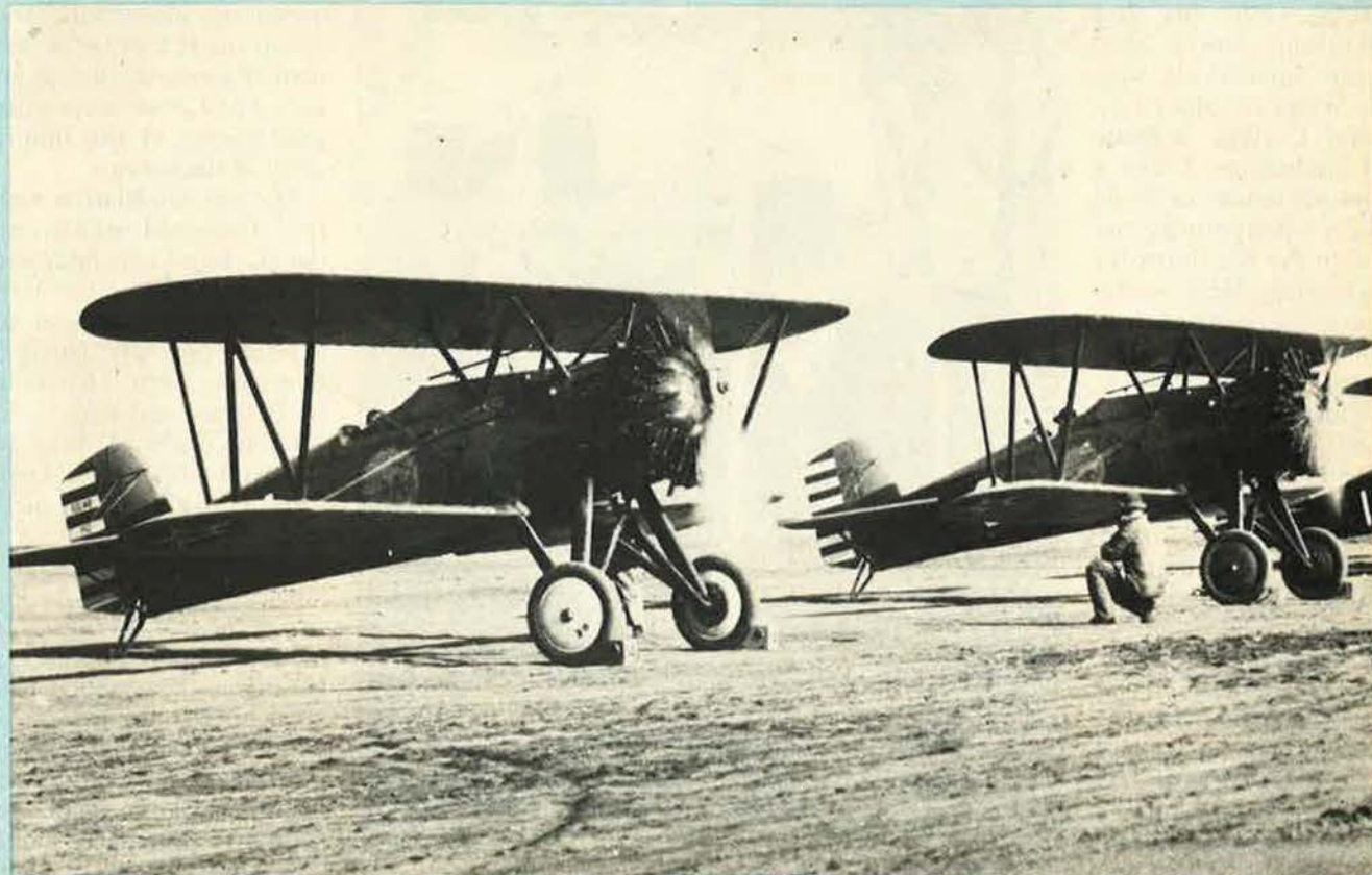
These early 95th Squadron P-12s had 450-hp P&W Wasp engines, a top speed of 170 mph, and a range of about 500 miles.
