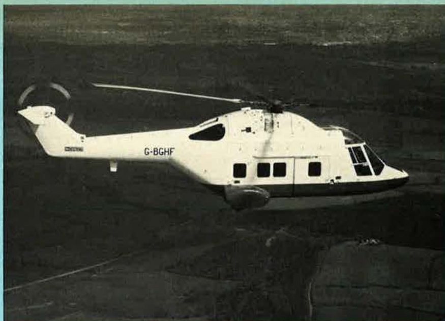
Westland's new WG 30 twin-turboshaft general-purpose helicopter, first flown on 10 April and intended as a Puma replacement
