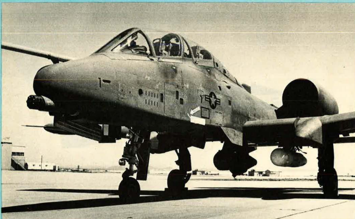
Fairchild Republic Night/Adverse Weather A-10, a two-seat version of USAF's Thunderbolt II
