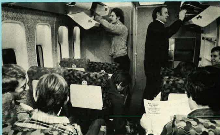
The cabin of the Model 234 Commercial Chinook, shown here in a display mockup, has window size and spacing identical to those of the Boeing 727
