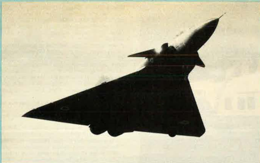
This view shows well the canard surfaces of the new twin-jet Dassault Super Mirage 4000
