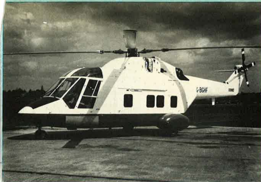
The WG 30 uses many already proven dynamic components of the successful Westland Lynx
