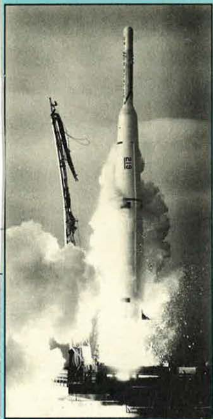
The US's first strategic missiles also became launch vehicles, like this Thor, for orbiting satellites.
