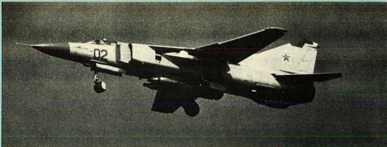
Armed usually with air-to-air missiles, this MiG-23S ('Flogger-B') of the Soviet Air Force carries two underbelly rocket pods ( Flug Revue )
