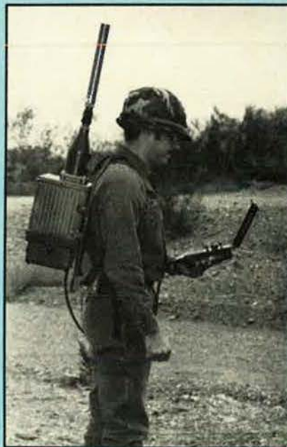
Navstar GPS signals received on these twenty-seven-pound backpacks enable soldiers to guide artillery accurately.
