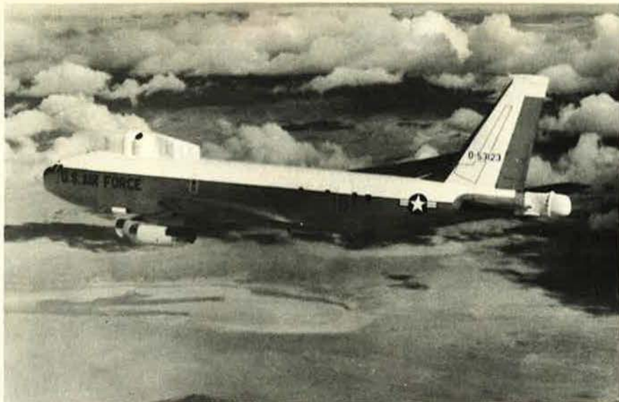
A new high-power, gas-dynamic laser, built by Pratt & Whitney, is under test aboard this NKC-135 Airborne Laser Laboratory at Kirtland AFB, N. M.
