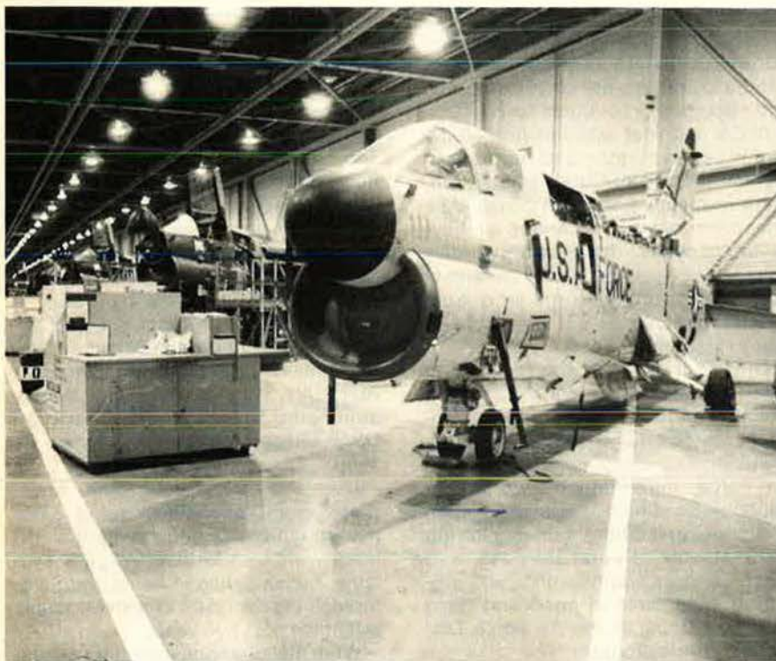
AFLC's Oklahoma City Air Logistics Center supports USAF's fleet of A-7Ds. This is part of the A-7D depot maintenance line at the Tinker AFB facility.
