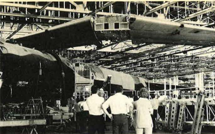
To extend the life of the D models, new skin panels for wings and fuselage, new leading and trailing edges for the wings, and new electrical wiring were added.
