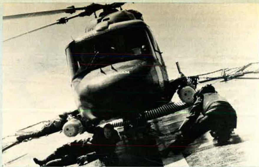
HMS Birmingham's Lynx helicopter proves its ability, with harpoon engaged, to remain securely fixed to a steeply rolling deck
