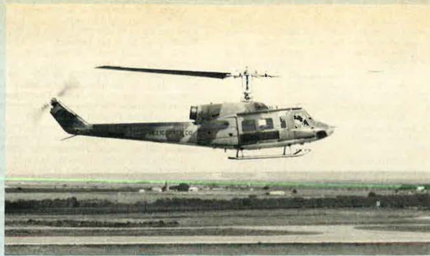
Largest glassfibre rotor blades yet flown being tested on a Bell Model 214
