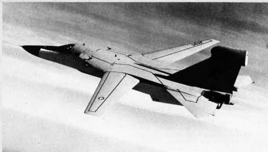
Second prototype of the EF-111A, modified by Grumman from a standard F-111A
