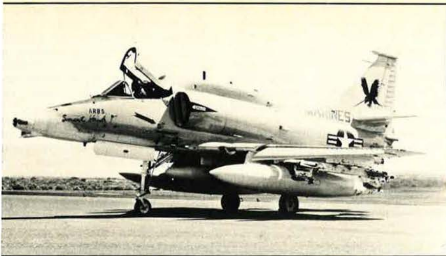
A new Angle Rate Bombing System (ARBS), whose "eye" can be seen mounted in the nose of this A-4M, is expected to sharply improve the day and night accuracy of these Marine Corps attack aircraft. The plane participated in the evaluation of the weapon aiming and delivery system developed by Hughes Aircraft Co.
