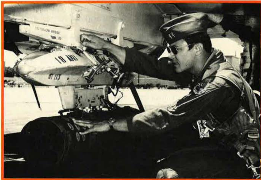
The RF-4C rocket pod carries seven 2.75-inch white phosphorous rockets used to mark targets. A strike aircraft, following shortly behind the reconnaissance aircraft, uses the rockets' white cloud to fine-tune ordnance delivery.
