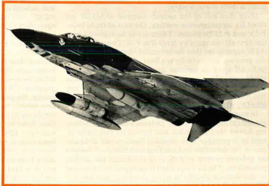
RF-4Cs, equipped for Quick Strike Reconnaissance, can locate and identify targets, relay their location to an interpretation center, stand by until tactical fighters arrive, and then pinpoint the target with a laser beam.
