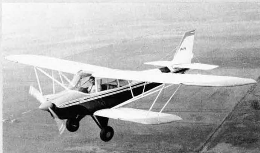
Aero Boero 180 SP agricultural aircraft is unique in having added biplane wings to house its chemical tanks
