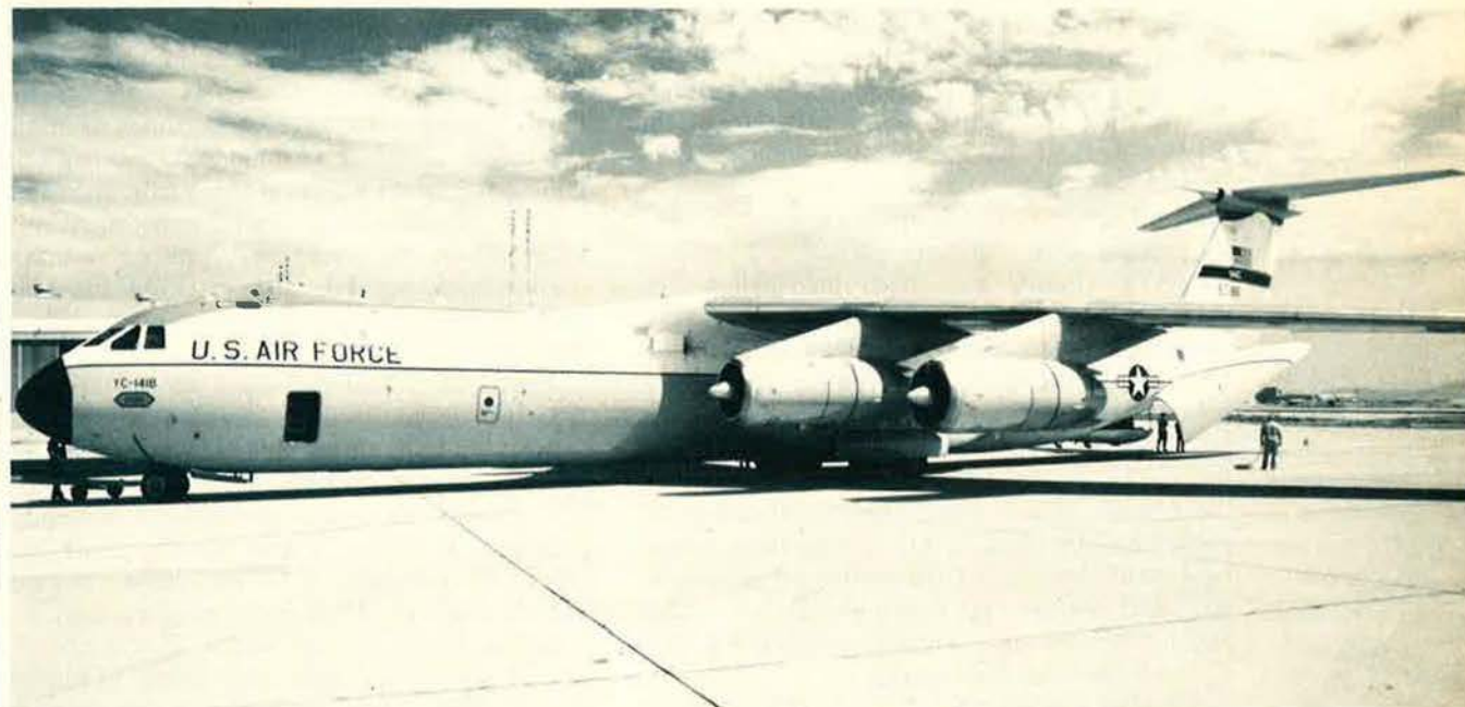
Above, a “stretched” C-141 (YC-141B), one of such planes that will add substantial airlift capacity to MAC’s fleet of strategic transports. For strategic airlift, MAC relies on its force of some seventy C-5s and 230 C-141s like the aerial workhorses, right, shown at Rhein-Main AB in Germany.
