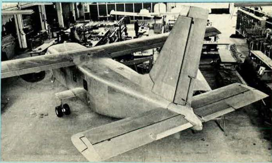
General Avia F.600 Canguro prototype, nearing completion in Milan
