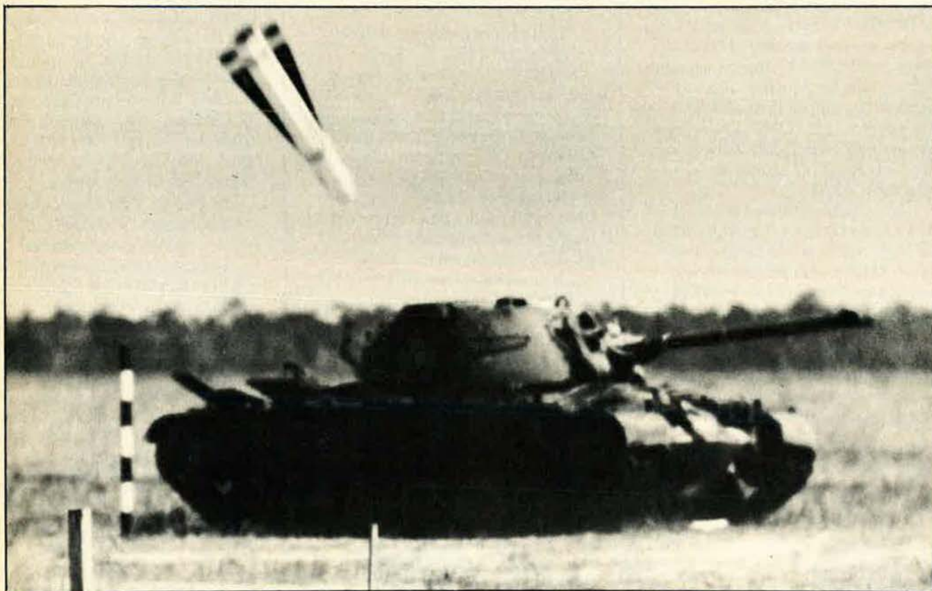
A laser-guided Maverick—the latest version of Hughes Aircraft Co.'s air-to-surface missile—an instant before direct hit on a tank. In a recent series of test launches, the weapon exceeded the reliability record set by earlier Mavericks.
