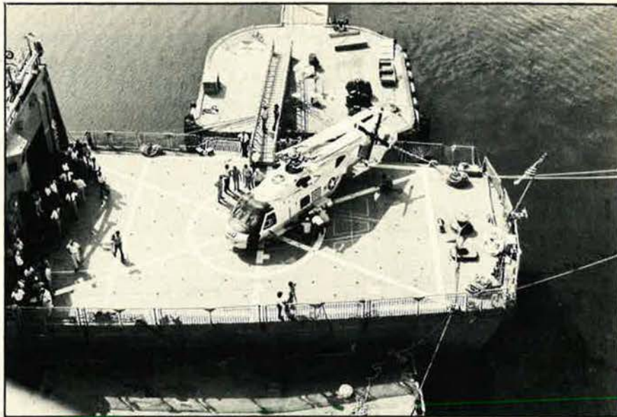
A mockup of the new Sikorsky SH-60B anti-submarine warfare helicopter during recently completed shipboard compatibility trials. Joining the fleet in the mid-'80s, the SH-60B will operate from Navy frigates and destroyers.
