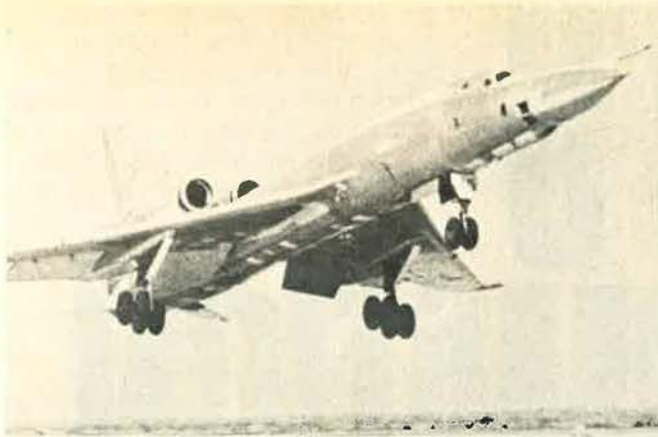
First supersonic (Mach 1.4) Soviet bomber was the 1,400-mile-range Tu-22 Blinder, first shown in 1961.
