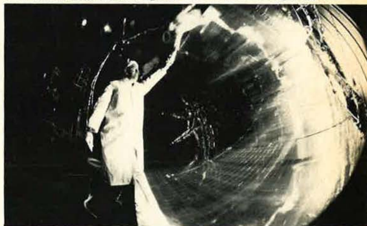
Space Shuttle Radiator in the environmental test chamber.
