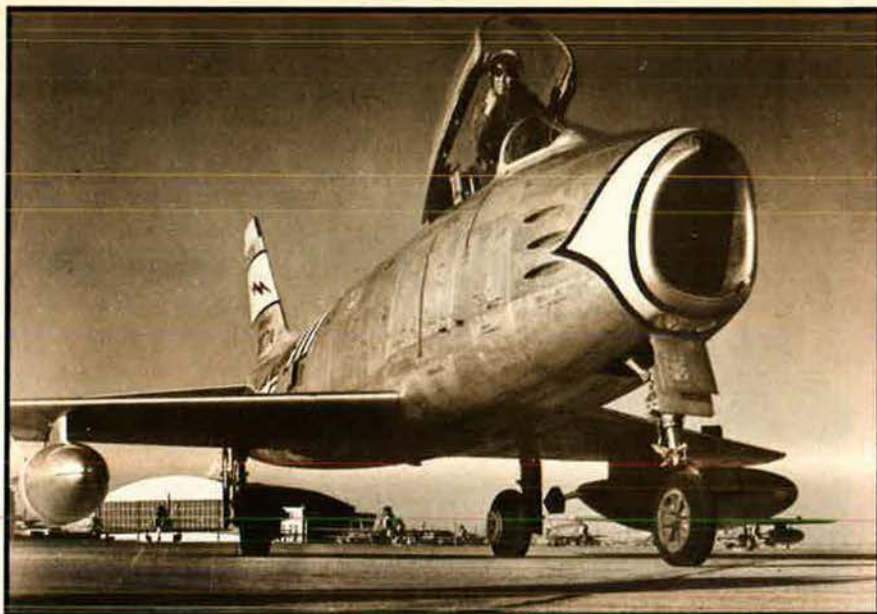
Bigger, wider, heavier, and faster than its predecessors was the F-86H, final production version of the Sabre. It was powered by the J73-GE-3 engine, an improved version of the J47. USAF received a total of 473.
