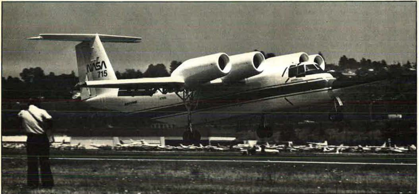
Taking off on a first flight this past summer is a de Havilland of Canada Buffalo extensively modified by NASA as an experimental Quiet Short-Haul Research Aircraft. See item below for details.
