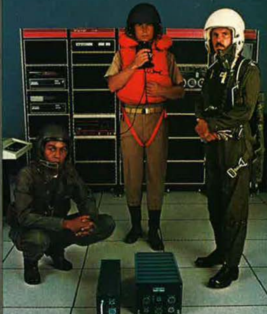
PDP-11/34M. Medium sized minicomputer with modular core memory from 16K to 128K words in increments of 16K and 32K words plus all standard operating features of commercial PDP-11/34 system. CACHE memory available as plug-in, double card module that boosts throughput up to 100%. Hardware floating point processor also available.
