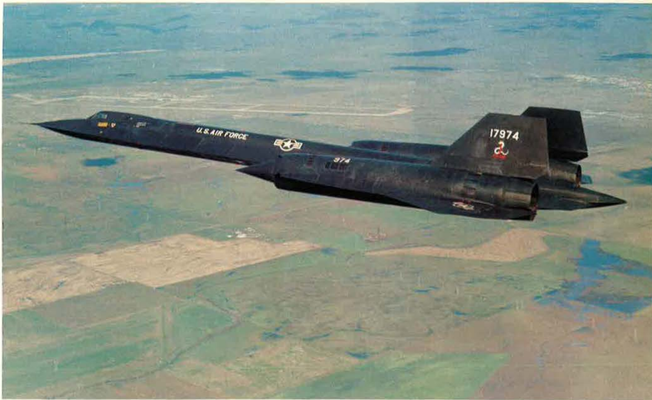
SAC's high-performance SR-71 reconnaissance aircraft, capable of operating at three times the speed of sound, is a candidate for upgrading.
