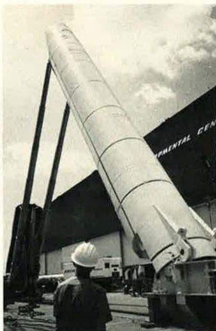
Left: Experimental transporter/launcher for MX at Boeing Developmental Center. Below: Artist's concept of MX horizontal shelter, one multiple-aim-point approach under study.
