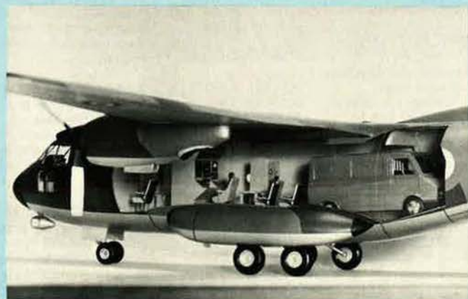
Interior layout of flight inspection version of Aeritalia G222
