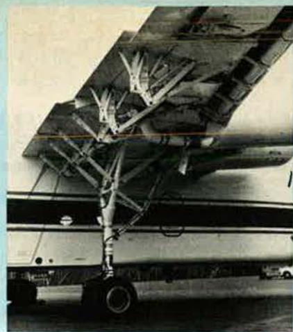
Close-up of the flap mechanisms and engine bleed air cross-ducting under the starboard wing of the QSR4. No attempt was made at streamlining, as this would not affect the data required from the programme
