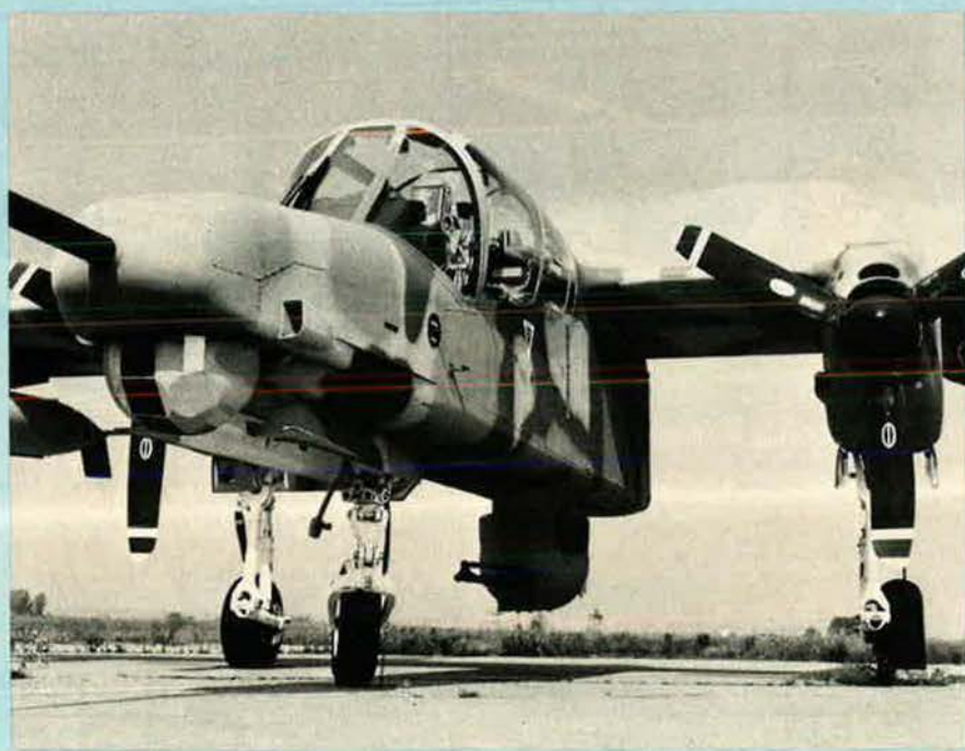
The YOV-10D has a 20 mm gun turret mounted beneath the aft fuselage
