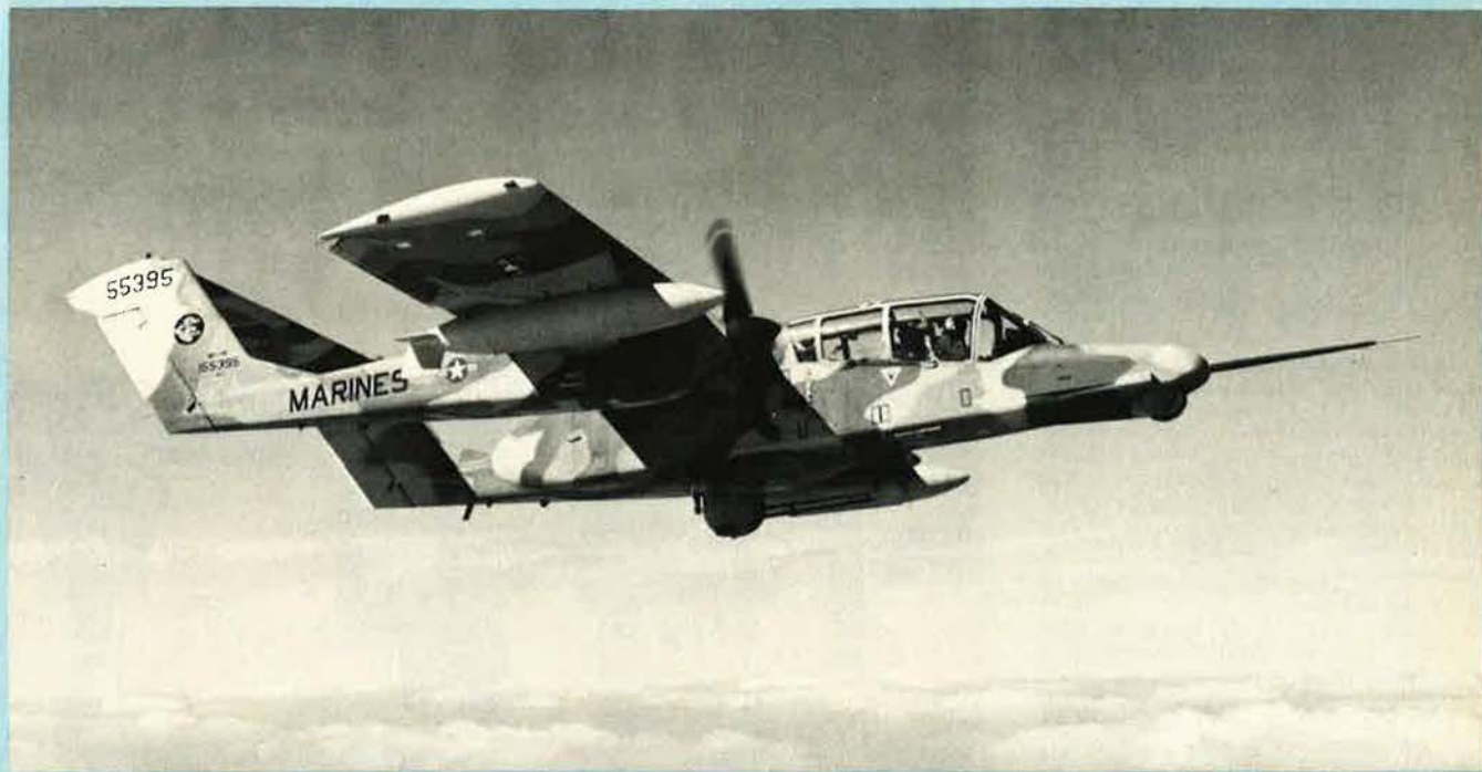
Pre-production Rockwell International OV-10D night observation surveillance aircraft (NOS) for the USMC
