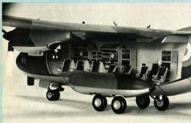
Model showing cabin layout of G222 equipped for electronic warfare
