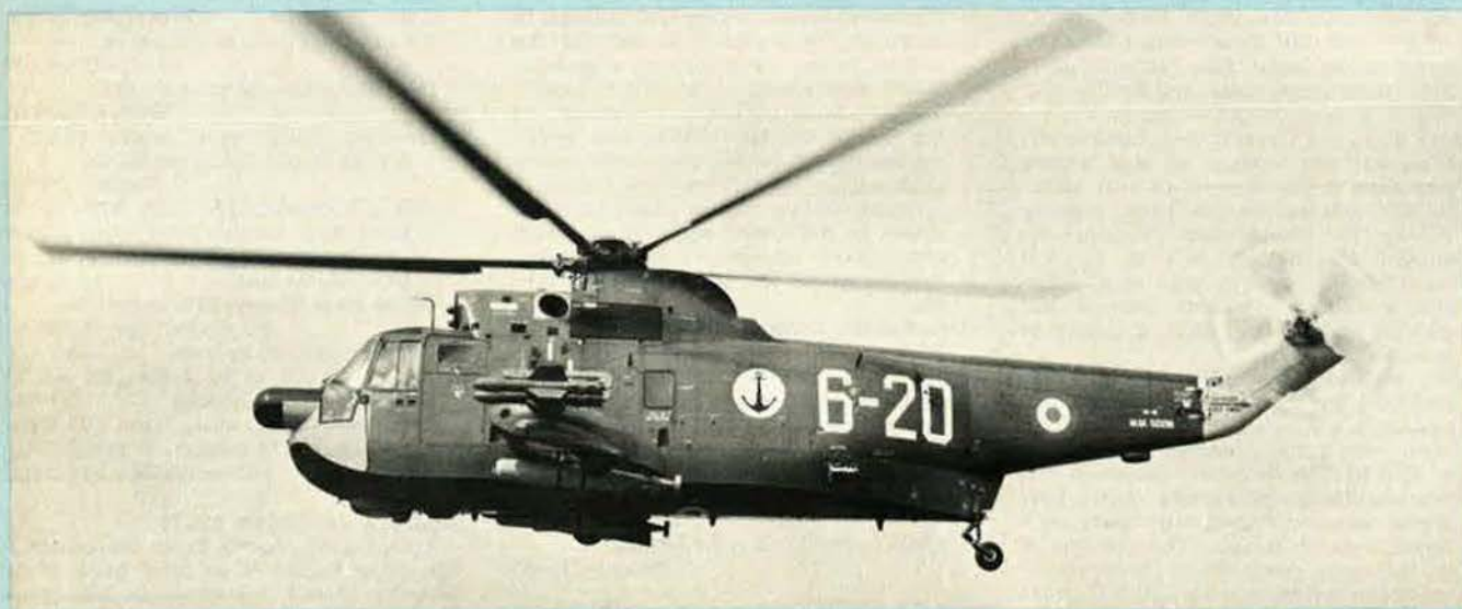
Agusta-Sikorsky SH-3D ASW/ASV helicopter, armed with two homing torpedoes and four AS.12 air-to-surface missiles
