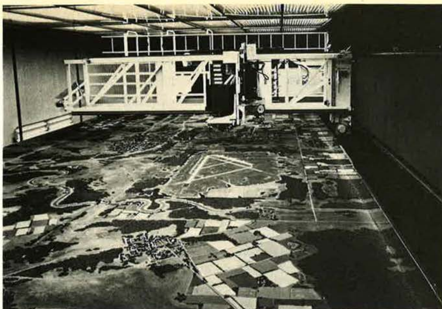
A television camera, above, responds to student pilots at a flight simulator's controls, passing over a model board to create the illusion of flight, shown at right.
