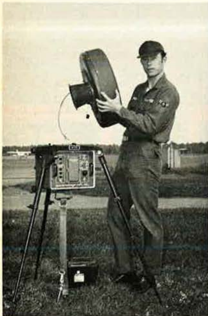
ESD's mini-TACAN can transmit bearing and distance information over a seventy-five-mile range.
