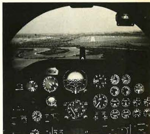
A television camera, above, responds to student pilots at a flight simulator's controls, passing over a model board to create the illusion of flight, shown at right.
