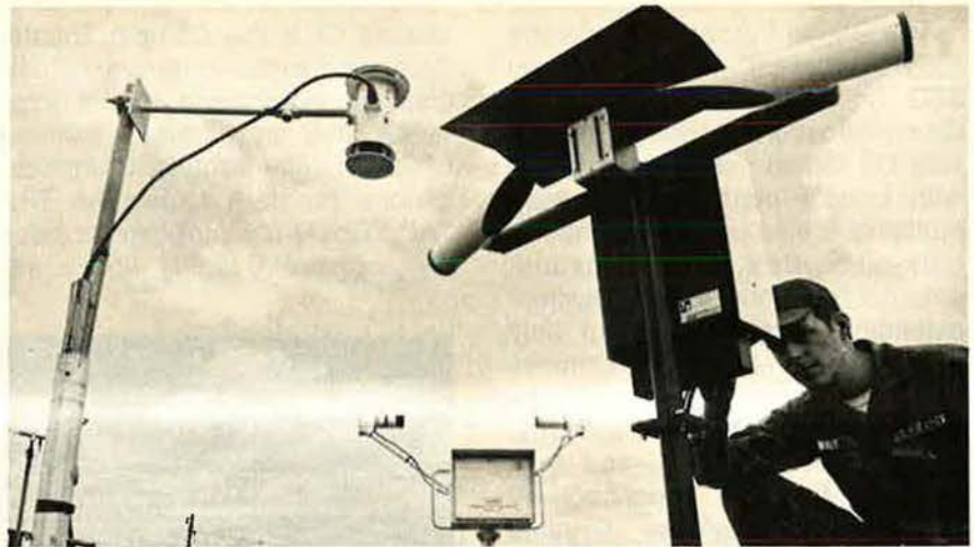
AFGL's Modular Automated Weather System uses microprocessors for short-range predictions of conditions critical to takeoff and landing.
