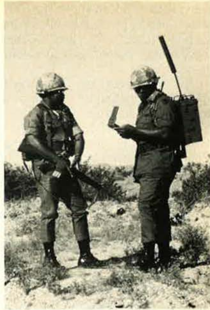
Army troops will be able to get from Navstar a position accurate to within fifty feet, using a manpack that weighs about twelve pounds.
