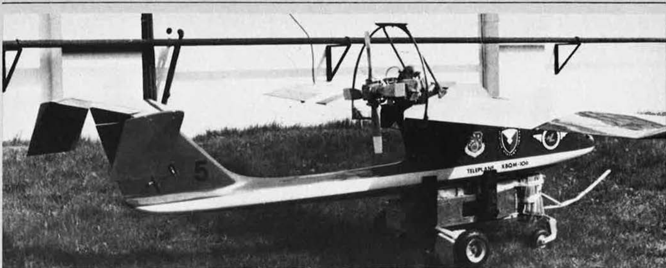
Ram-air canopy experimental version of the XBQM-106 mini-RPV on its take-off dolly
