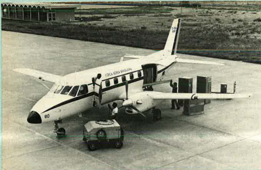
The Brazilian Air Force's C-95A is an EMB-110K1 all-cargo version of the Bandeirante
