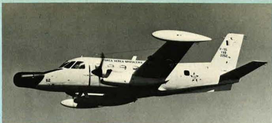
With AIL search radar in its nose, the EMB-111 is a specialised coastal patrol development of the basic Bandeirante
