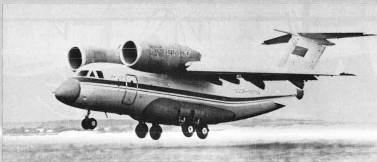
Prototype of the Antonov An-72 twin-turbofan STOL transport (Tass)
