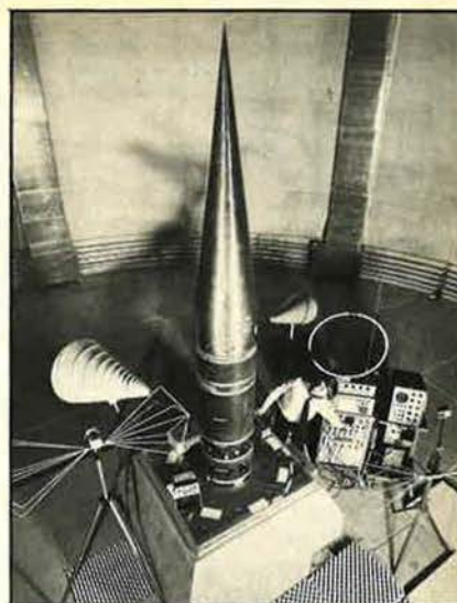
British Skylark research rocket gets going-over in the electromagnetic "clean room" at a British Aerospace facility in southwest England. Adjacent is "probably the best and most up-to-date computer data acquisition and analysis equipment anywhere in the world," the firm said.
