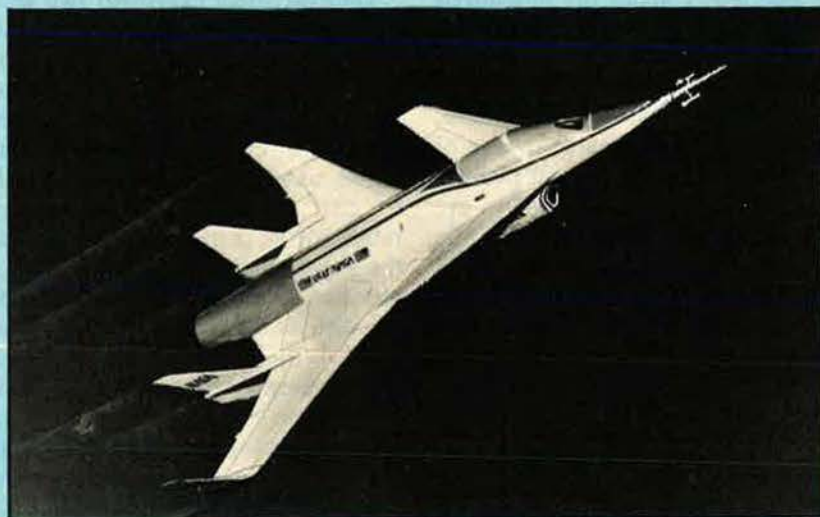
HIMAT, a remotely piloted vehicle about one-third the size of a fighter, will be a flying test-bed for new, sophisticated aerodynamic designs.
