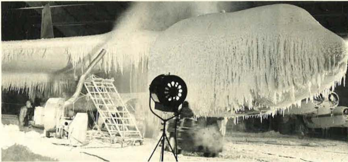
A B-52 undergoing cold-weather tests at AFSC's McKinley Climatic Laboratory, Eglin AFB, Fla., the world's largest environmental test chamber.
