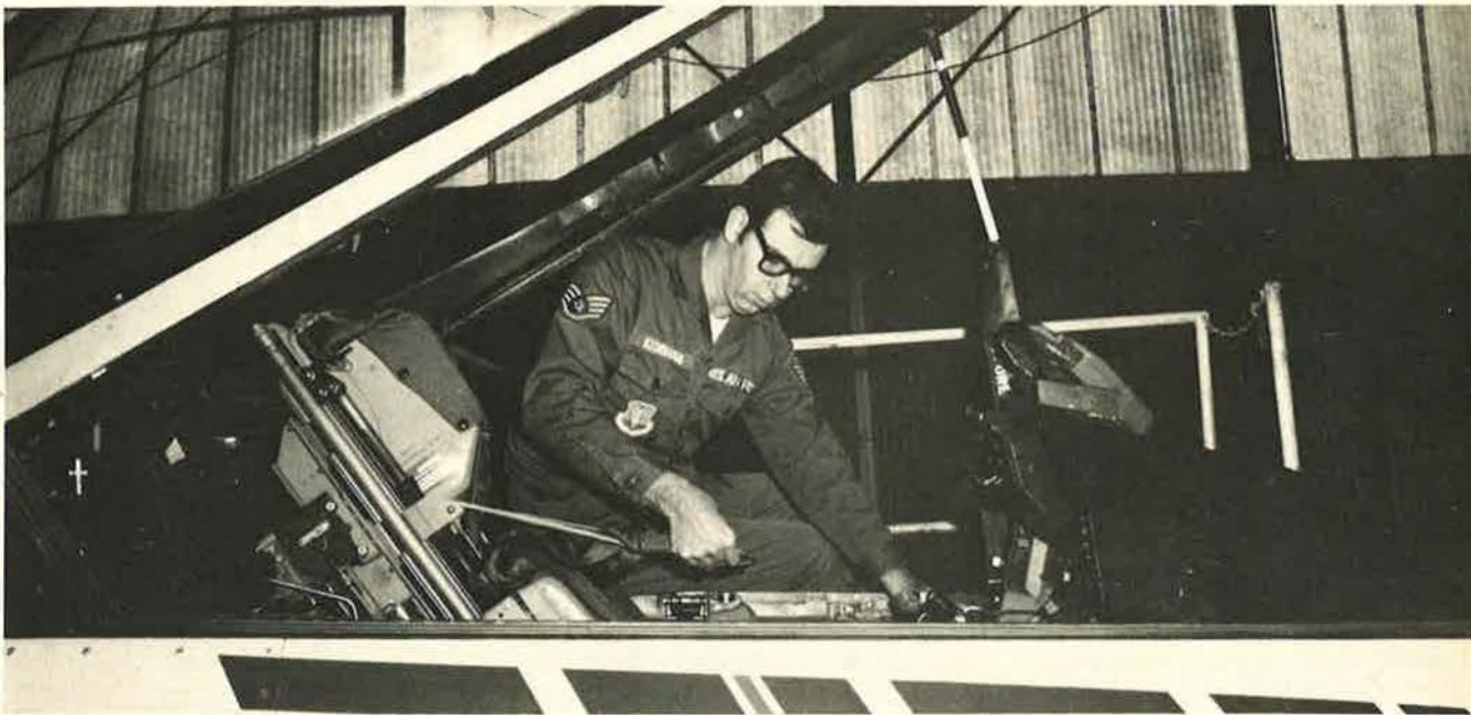
SSgt. Robert Kishbaugh, an F-16 egress specialist with the AFTEC F-16 Test Team, here works on the inertial reel of an F-16's ejection system.
