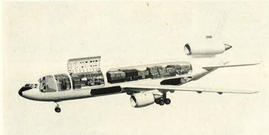
Artist's concept of the McDonnell Douglas DC-10 tanker/cargo aircraft that, in the 1980s, will enhance SAC's ability to support general-purpose forces.
