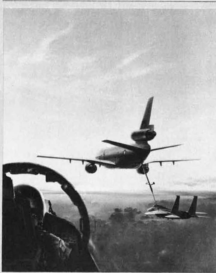
Artist's impression of the McDonnell Douglas Advanced Tanker/Cargo Aircraft flight refuelling an F-15
