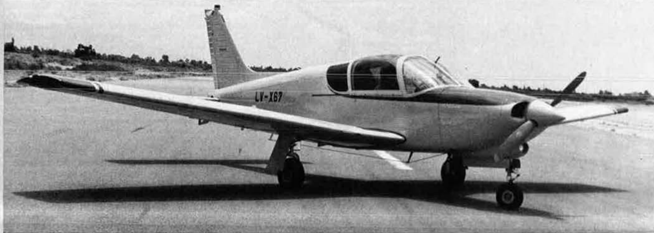
Prototype of the two-seat aerobatic military trainer developed by Chincul from the Piper Arrow lightplane
