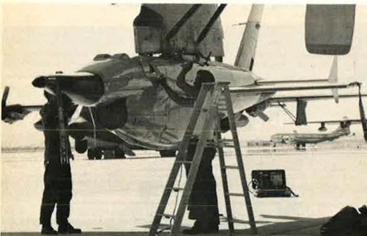
Top, note DC-130A's chin dome, housing microwave command guidance system (MCGS). Above, members of 432d Drone Generation Squadron "button up" an AQM-34M drone.
