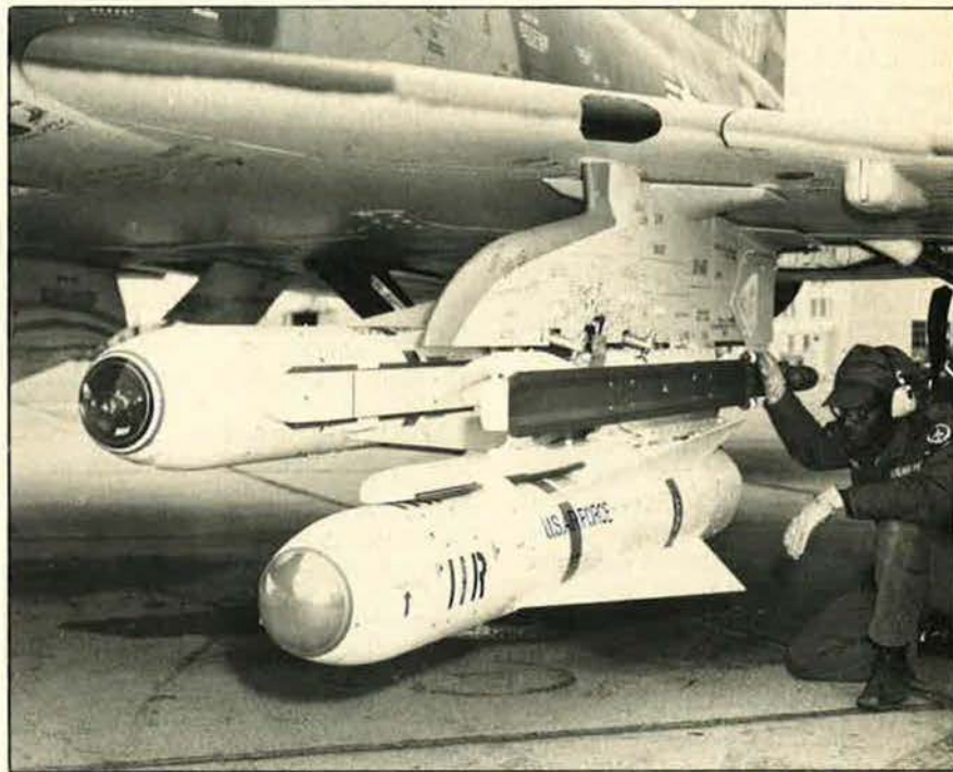
Recent flight tests have verified that this new imaging infrared seeker can accurately discriminate targets through darkness, smoke, or low-visibility haze. Developed by Hughes Aircraft Co., the seeker gives Maverick missiles night capability in close support and interdiction missions.
