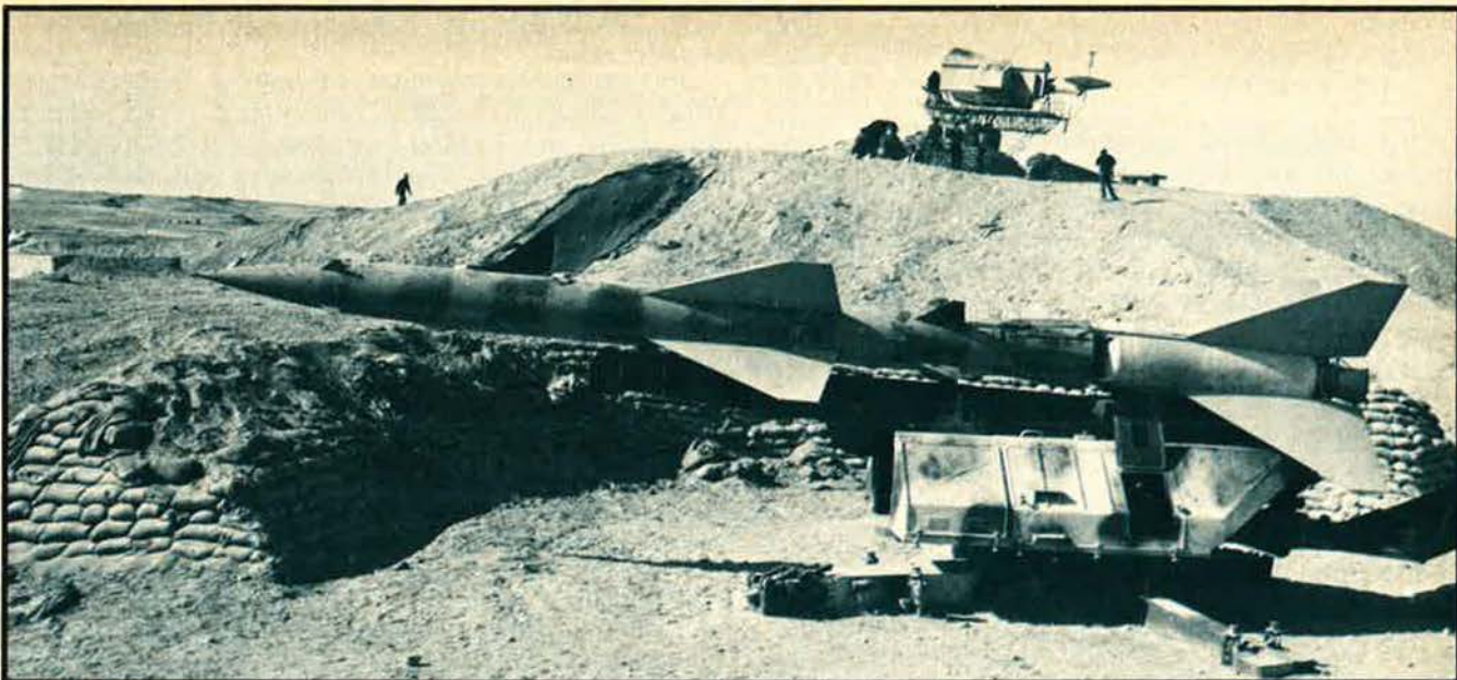
SA-2 Guideline with Fan Song radar is one of a number of anti-aircraft missiles deployed in the USSR and the Pact area.
