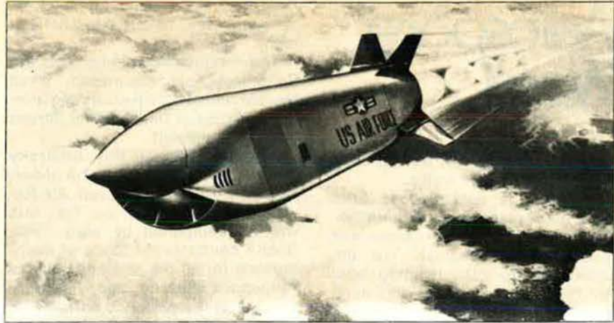
Artist's concept of the Advanced Strategic Air-Launched Missile being developed for USAF by McDonnell Douglas Corp. Supersonic, it will be powered to air or ground targets by an integral rocket ramjet propulsion system.
