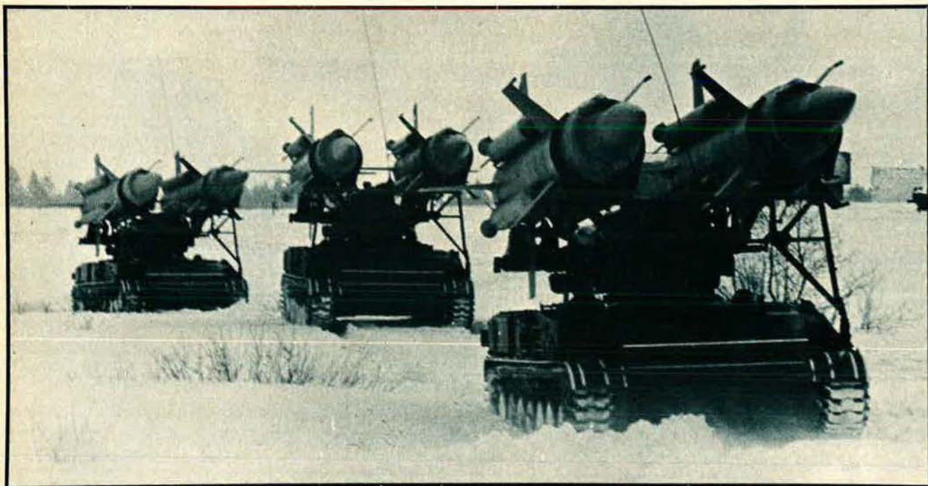
The SA-4 Ganef has the longest range of any PVO SV system—about seventy km. It can be airlifted by the An-22 transport.
