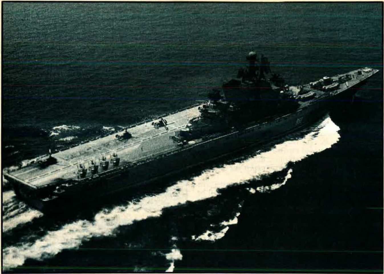
Though not designed for intensive air operations, the Kiev can carry up to thirty-six V/STOL fighters and ASW/electronics helicopters.
