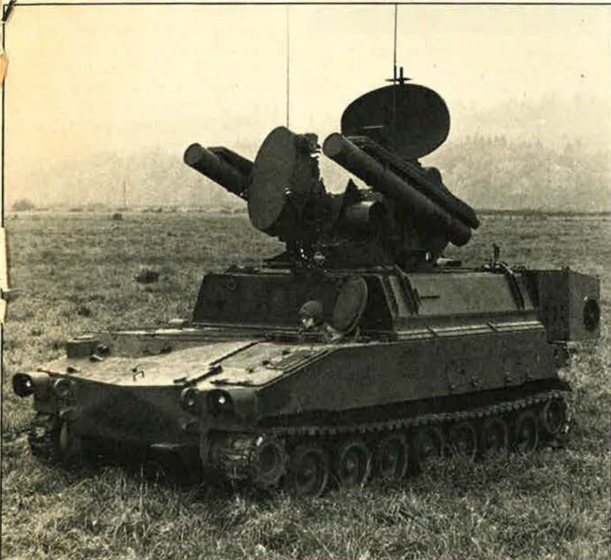
Above, short-range Roland missile system designed to down ground-hugging aircraft, mounted on M-109R tracked vehicle. Right, cutaway view of missile.
