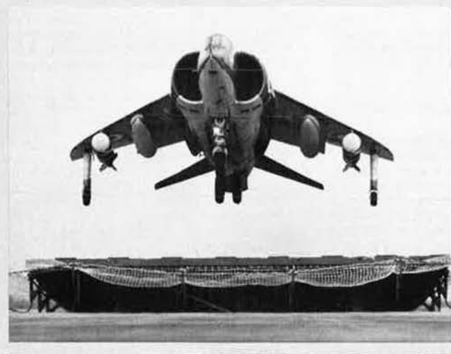
Single-seat Harrier XV281 leaving the 6° ramp with two 455 litre (100 Imp gallon) fuel tanks and two BL755 cluster bombs underwing
