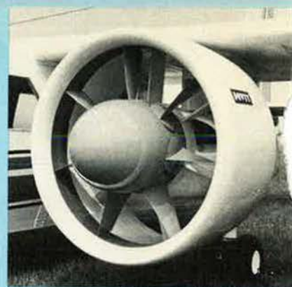
Close-up of one of the seven-blade Ducted Propulsor units fitted to Islander G-FANS
