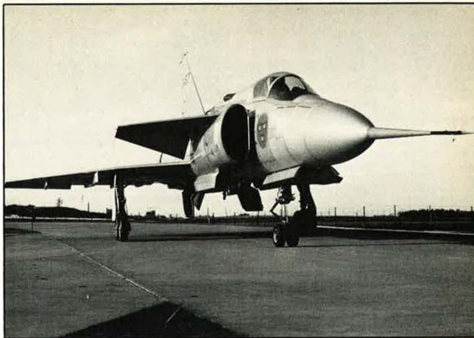
With 504 home-built combat aircraft, Sweden has the third largest air force in noncommunist Europe. This Mach 2 Saab-37 is adaptable to fighter, support, or recce roles.
