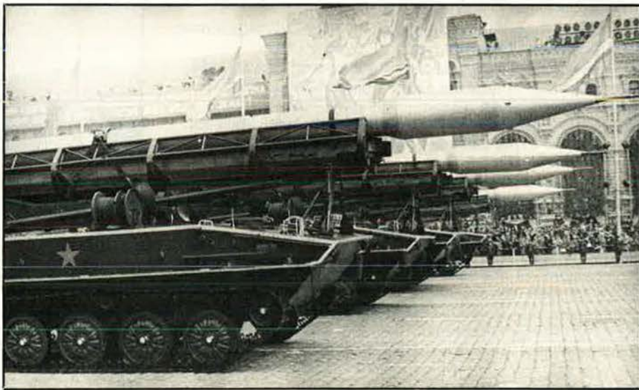
All Pact armies are equipped with FROG surface-to-surface missiles. This obsolescent FROG-3 is dual-capable and has a range of about forty kilometers.
