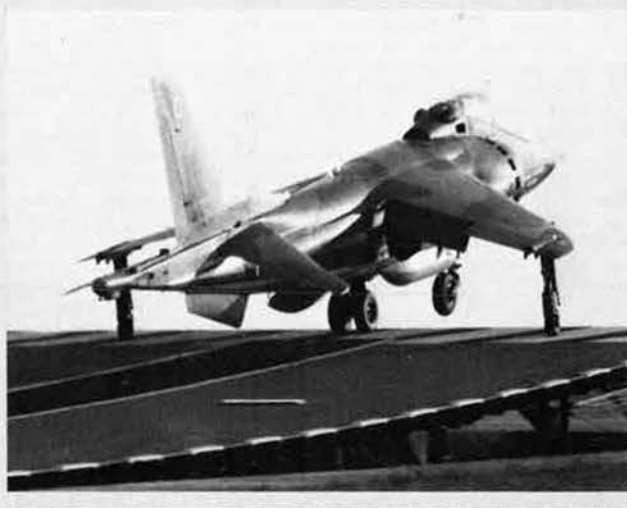
RAE Bedford's own Harrier T.Mk 2A two-seater, XW715, leaving the 6° ramp during initial ski jump trials
