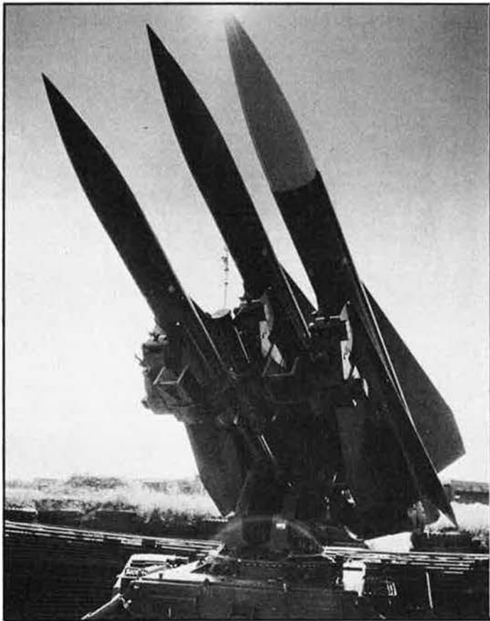
US-built HAWK surface-to-air missiles, effective at altitudes from 30 to 11,000 meters, are used by seven NATO military forces.
