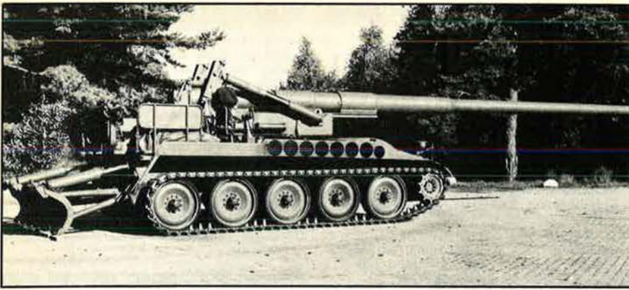
This 175mm self-propelled gun, developed by the US Army, is used by the UK, Turkey, the Netherlands, and Germany. It fires only HE rounds and has a range of 32,700 meters.
