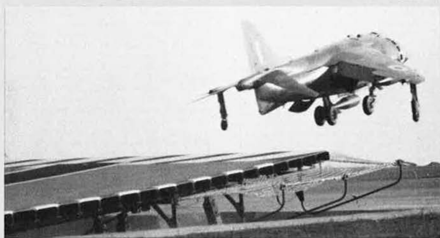
STOL take-off with three 1,000 lb bombs by Harrier XV281 from the 6° ski jump ramp at RAE Bedford (see next page for item)
