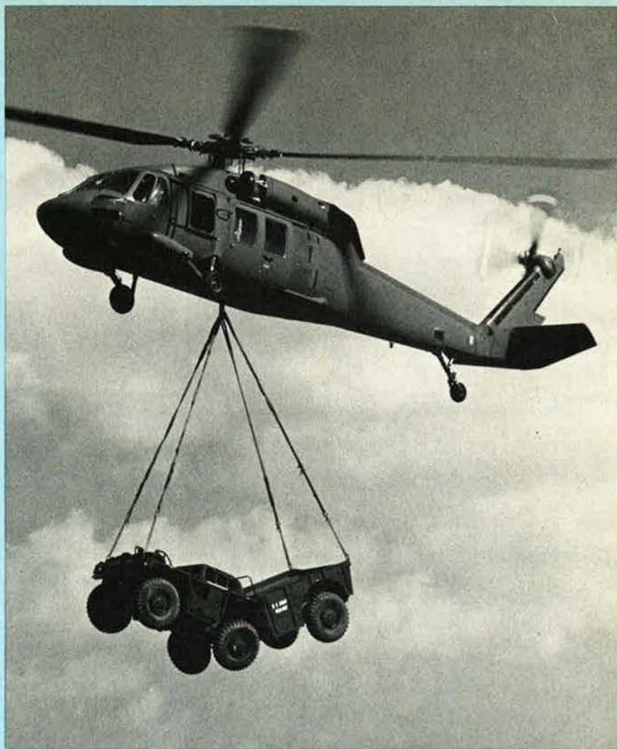
Max payload of the UH-60A Black Hawk in a flying crane role is 3,630 kg (8,000 lb)
