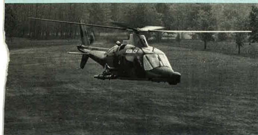
The TOW-equipped anti-armour version of the Agusta A 109 for the Italian Army. The naval version will be basically similar but will carry extensive armament and equipment for ASW, ASV, SAR, and other duties
