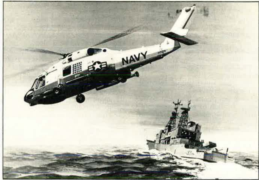
Artist's rendition of a sub-hunting Sikorsky LAMPS Mk III helicopter flying from a US Navy vessel. LAMPS capability would include RAST—for Recovery Assist, Secure, and Traverse—making operations from smaller ships possible.
