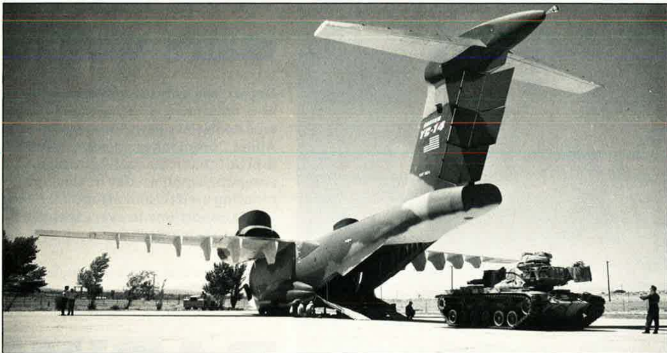
Loading and clearance tests of an M-60 main battle tank aboard a Boeing YC-14 Advanced Medium STOL aircraft were recently conducted at Edwards AFB, Calif. Boeing engineers calculate that a C-14 production version could airlift a combat-ready M-60 some 500 miles (805 km).
