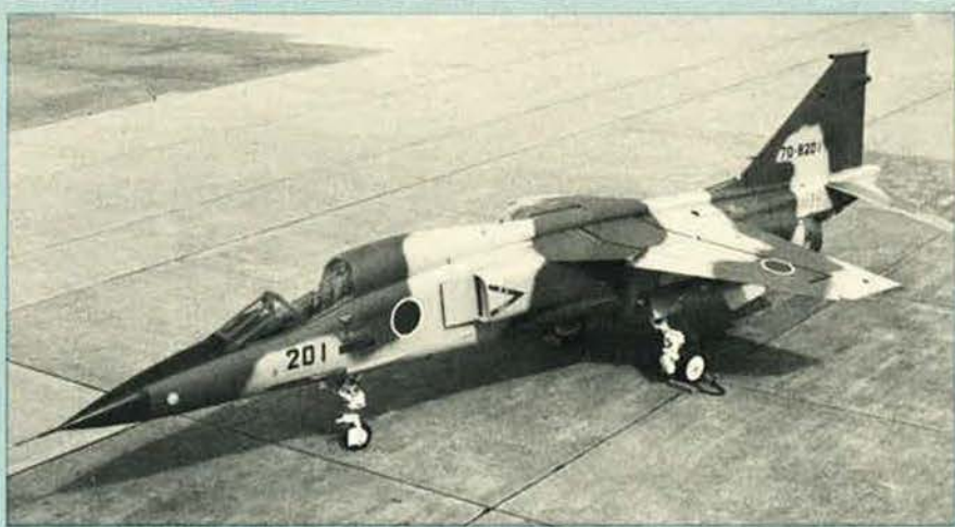
Mitsubishi F-1 single-seat close air support fighter, evolved from the T-2 supersonic jet trainer
