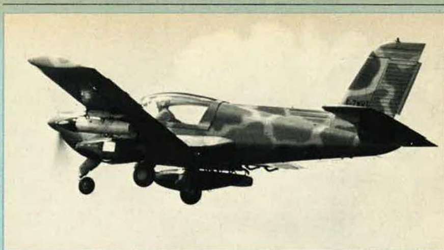
SOCATA Rallye 235 G in ground support configuration with underwing armament of two rocket packs and two gun pods
