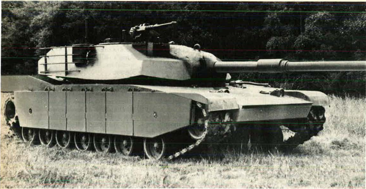
Chrysler Corp. has been named prime contractor for the new XM-1 tank, shown here in prototype. It is scheduled to enter the inventory in 1980. The XM-1 is only 92.5 inches high and has antitank-missile-repelling armor.
