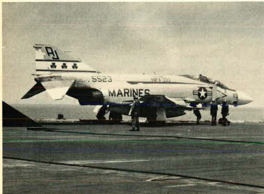
The Marine F-4J Phantom, identical to the Navy model, resembles the USAF F-4D but has wings and landing gear stressed for carrier operations.
