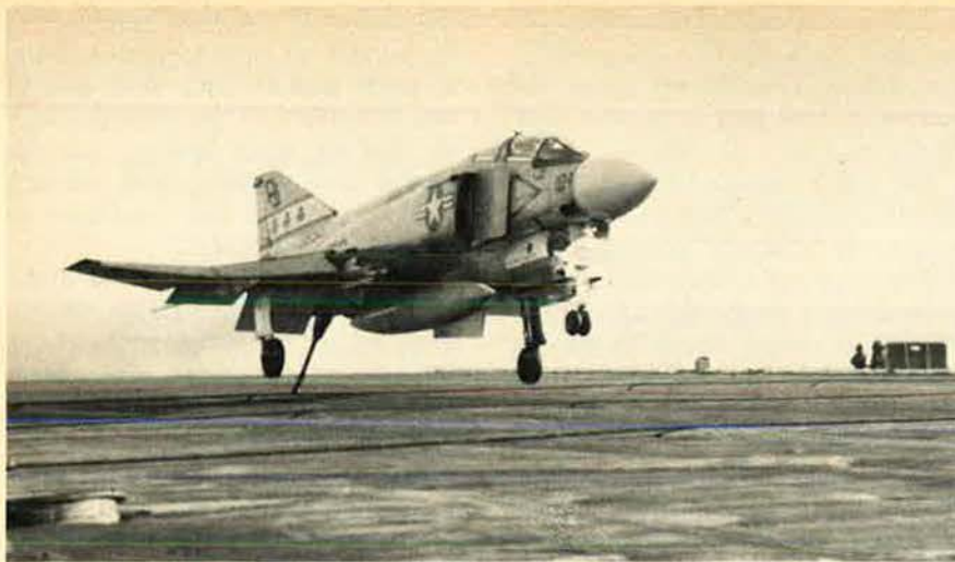
Descending about 750 feet per minute, a Phantom "traps" one of four steel cables located a third of the distance up one of Nimitz's two 700-foot decks. The "very violent" hookup halts the jet within three seconds.
