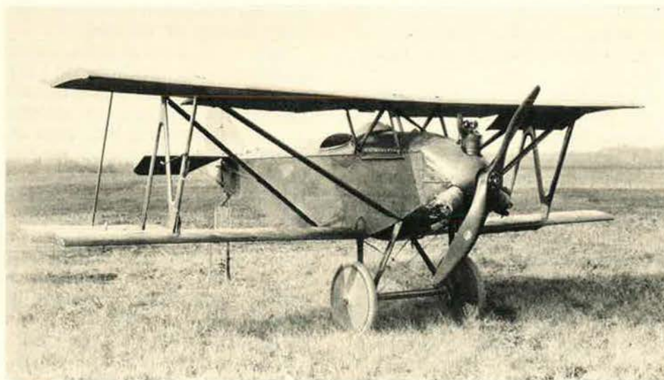
The Sperry Messenger was designed in 1921 at Wright Field, Ohio, and put on contract by the Air Service for Sperry to manufacture. The name "Messenger" came about after Gen. Billy Mitchell used it to deliver dispatches during Army maneuvers. About fifty of these vehicles were produced. Wright Field used it as a manned test-bed to continue the "aerial torpedo" experiments that had begun during World War I.
