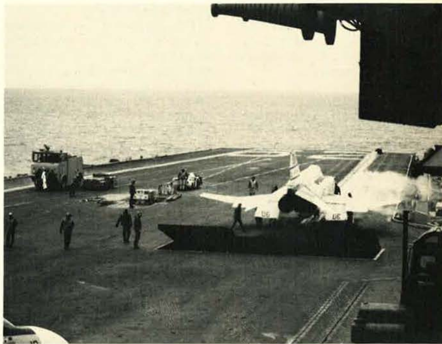
A Trip Trey Phantom readies for 300-foot launch from one of two steam-driven catapults on Nimitz's bow.
