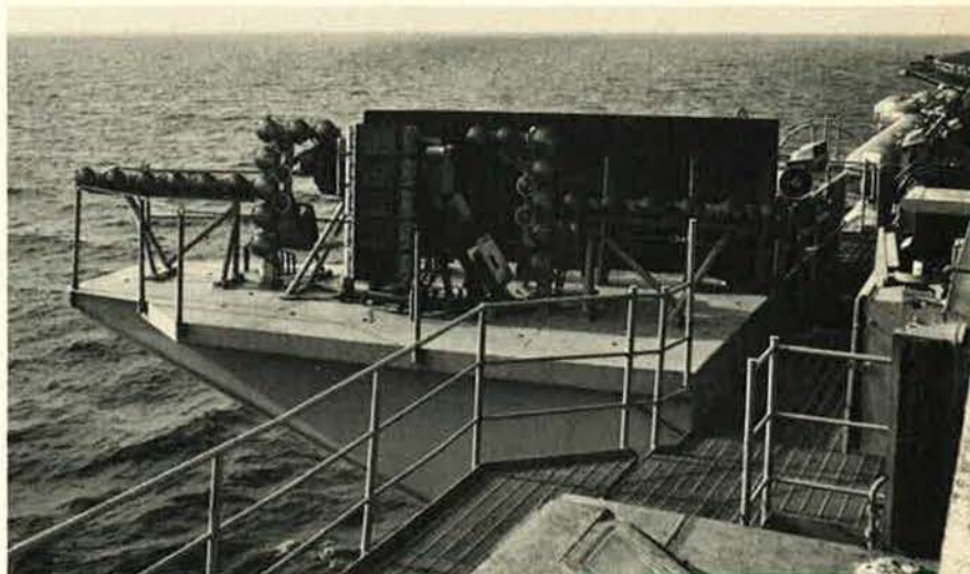
The "meatball"—center light on the Fresnel Lens Optical Landing System on port side of deck—shows pilot his approach position in relation to the desired glide path from two miles prior to touchdown.
