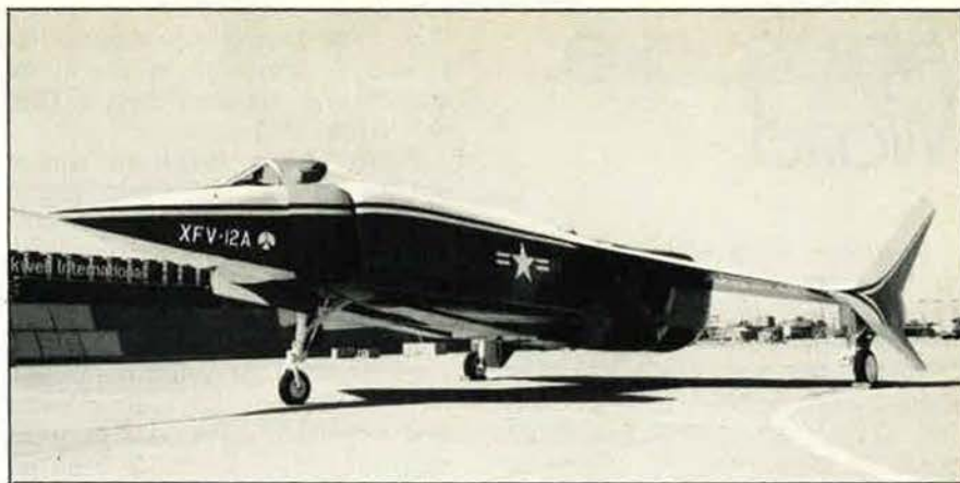
Rollled out recently was the Navy's new XFV-12A Thrust Augmented Wing (TAW) prototype aircraft designed for vertical takeoff and landing. The small, single-engine, single-seat aircraft generates vertical thrust by exhausting engine air through nozzles in the wings. The horizontal stabilizers, called canards, are set forward of the main wings and below the fuselage, slightly behind the cockpit. Rockwell International built the airframe, Pratt & Whitney the engine.
