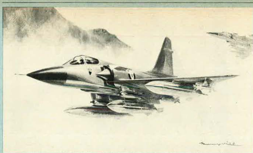
The projected strike version of the Mirage 2000 would carry 5 metric tonnes of external stores
