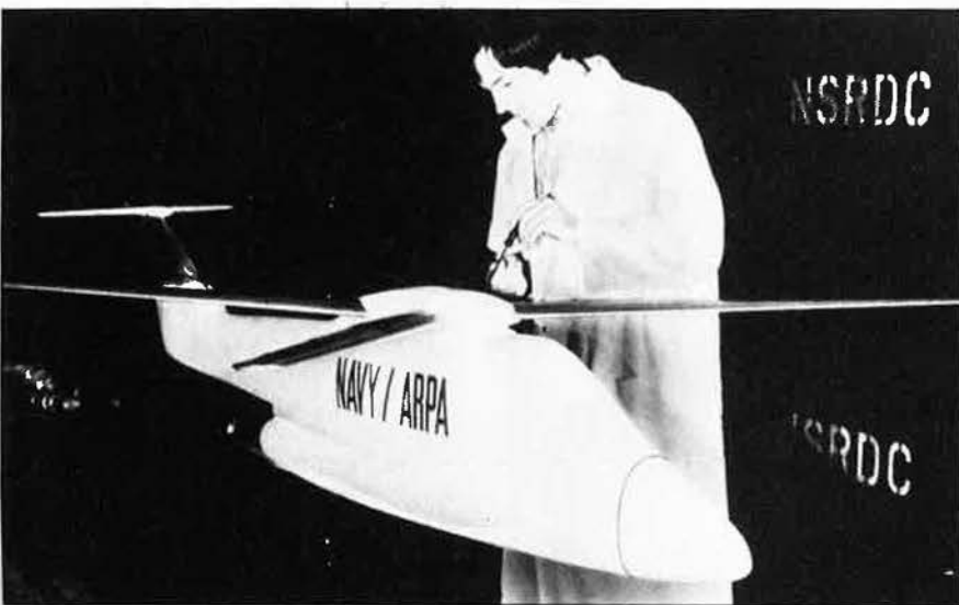
One-quarter-scale model of an X-wing experimental aircraft that could take off and land with wing rotating like a helicopter and fly conventionally with wing fixed. (See item below.)
