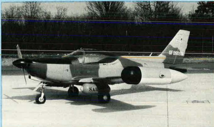
The new SIAI-Marchetti SF.260SW Sea Warrior, with Bendix radar in port wingtip pod, and underwing rescue pack
