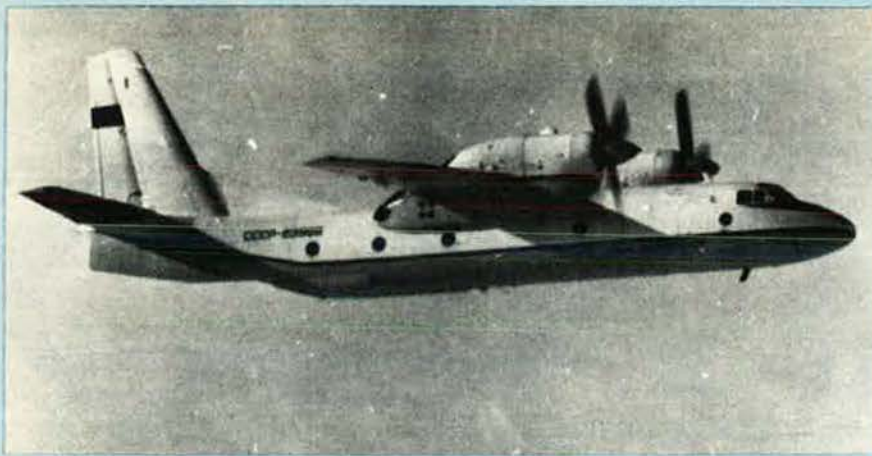
Antonov An-32, a new version of the An-26 transport with a major increase in engine power for take-off
