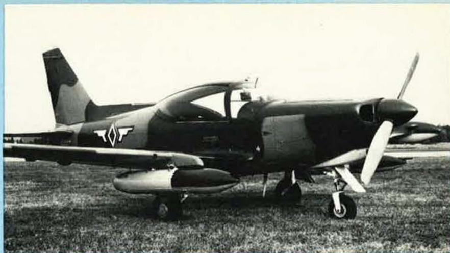
SIAI-Marchetti SF.260WP light strike aircraft of the Philippine Air Force, with underwing 7.62 mm gun pods
