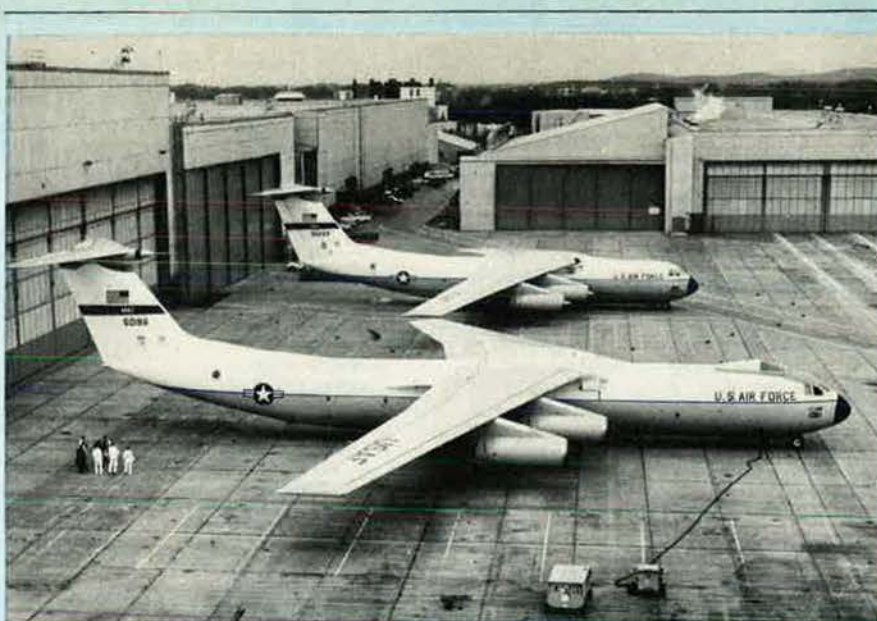
Prototype of the stretched Lockheed YC-141B StarLifter (foreground) beside a standard C-141. Overfuselage blister, aft of the YC-141B flight deck, is a flight refuelling receptacle
