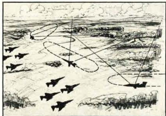
Above left: In the barrier standoff mission, EF-111As orbit near the FEBA, jamming early warning and other long-range surveillance radars. Above right: In the penetration escort mission, an EF-111A accompanies a strike force deep into enemy territory to cause confusion, delays, and loss of effectiveness in the enemy's air defense system. Right: The close air support mission brings the "Electric Fox" to the FEBA to suppress the enemy's air defense while the strike force carries out the attack.
