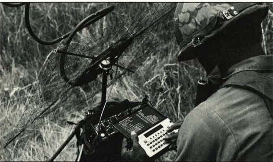
Capable of communicating over vast distances is this AN/PSC-1 manpack radio, the subject of recent testing. See item below.
