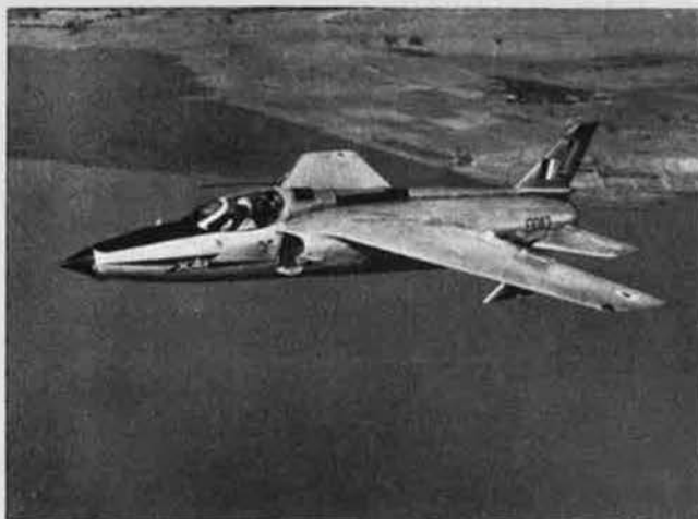
Prototype Ajeet lightweight combat aircraft, developed by HAL from the Hawker Siddeley Gnat
