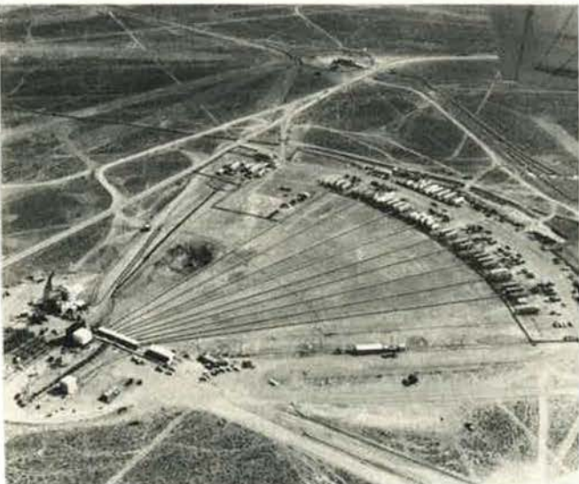
This aerial photo shows the array of equipment used at the Nevada Test Site during an underground nuclear test. The detonation point was hundreds of feet below the convergence of the signal cables that lead to recording instruments in the trailers at right. Surface settling from a previous underground detonation is visible at left of center.
