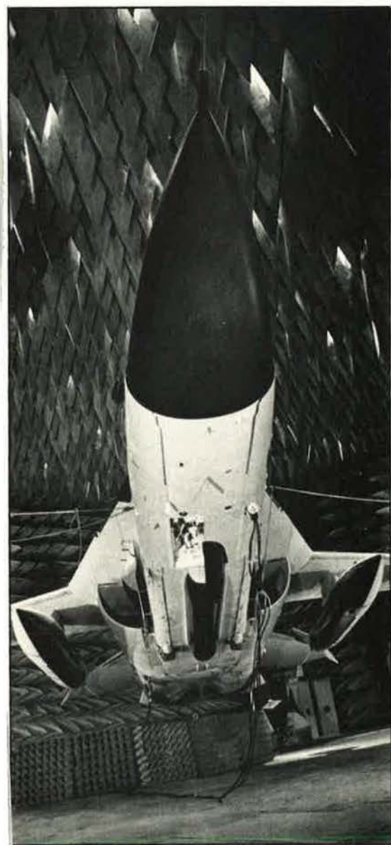
Full-scale tests in DoD's shielded anechoic chamber located at Grumman's Calverton facility (the world's largest) confirmed the electronic compatibility of the EF-111A's various electronic subsystems.
