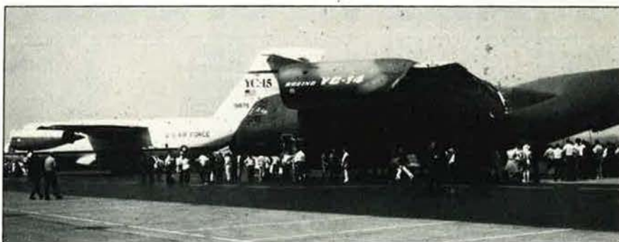
Together for the first time at Wright-Patterson AFB, Ohio, are the McDonnell Douglas YC-15 and Boeing's YC-14, contenders in USAF's Advanced Medium Short Takeoff and Landing (AMST) program. Both then headed for Europe.
