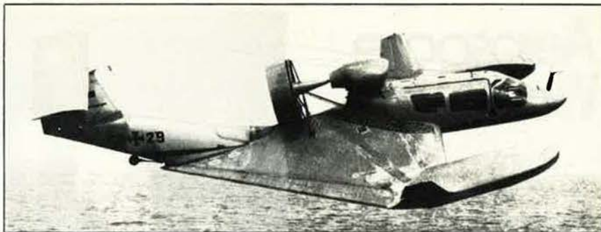
Tested successfully in the Baltic recently was this experimental X 114, a ground-effect craft developed by a VFW-Fokker subsidiary, Rhein-Flugzeugbau. The vehicle promises both civil and military applications.
