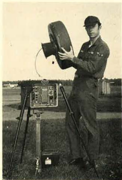
ESD's "mini-TACAN" for USAF Combat Control Teams can be air-dropped and transmits to aircraft within a seventy-five-mile range.
