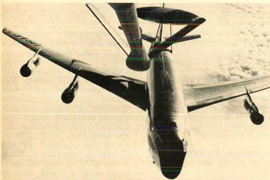
Already capable of long "on-station" operation, AWACS can increase its loiter time even further through aerial refueling.
