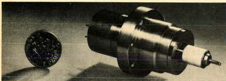
A Micro Electrostatically Suspended Gyro System utilizes a solid one-centimeter beryllium rotor spinning in a vacuum at 150,000 RPM.
