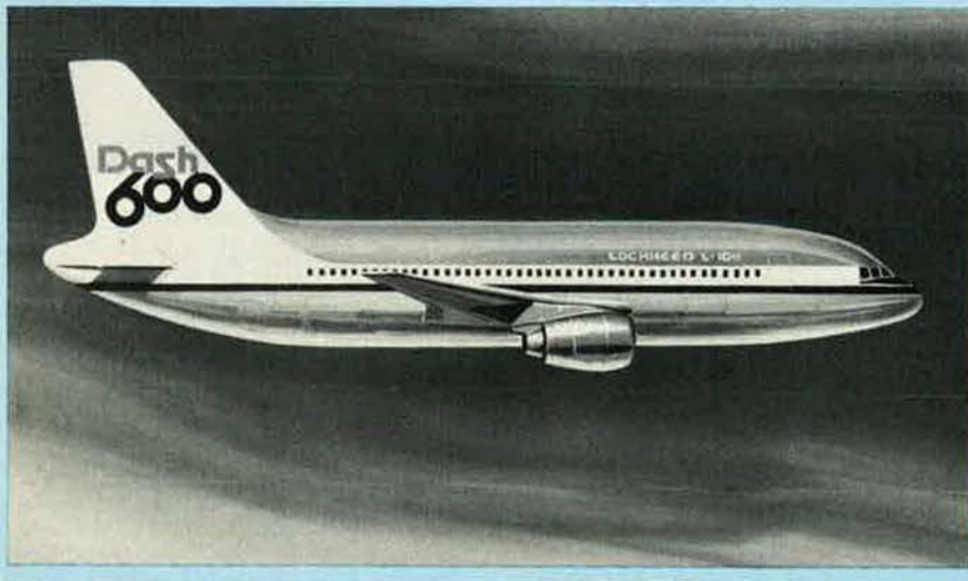
With two RB.211-524B turbofans, the L-1011-600 is Lockheed's projected 'compact' TriStar for the 1980s
