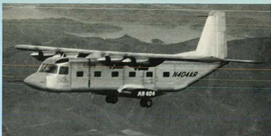
Prototype of the Ahrens AR 404, with non-retractable main landing gear and only six cabin windows on each side
