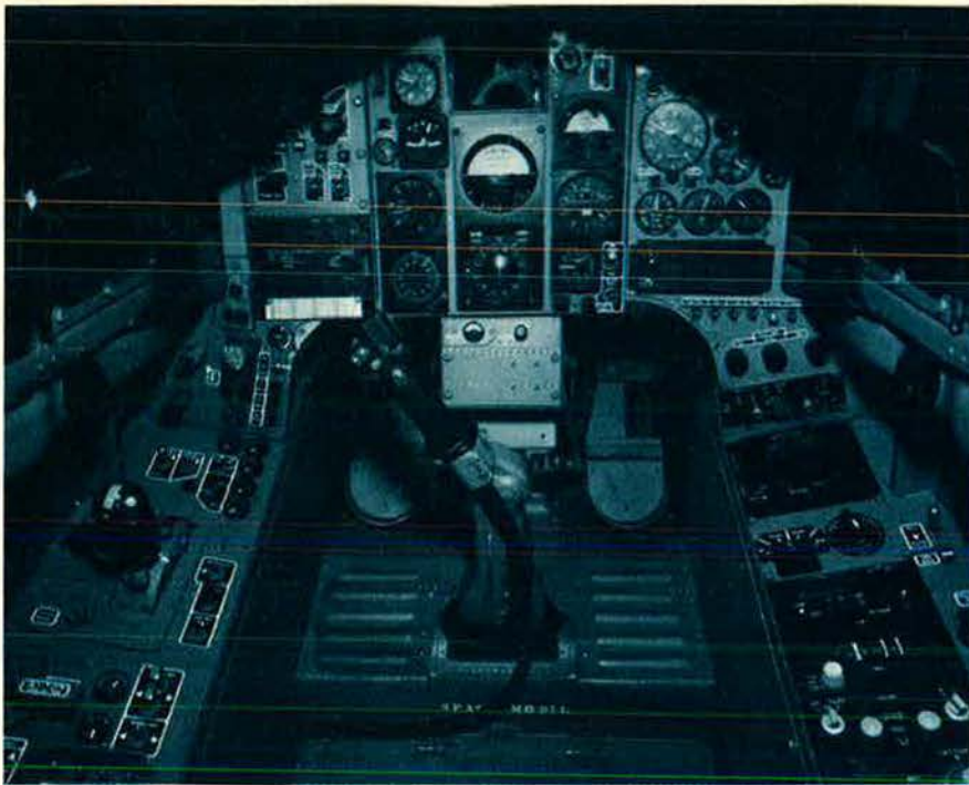
Hawk's cockpit is roomy, its layout designed with the pilot in mind. On the attack version, the weapons sight is above the Attitude Direction Indicator.
