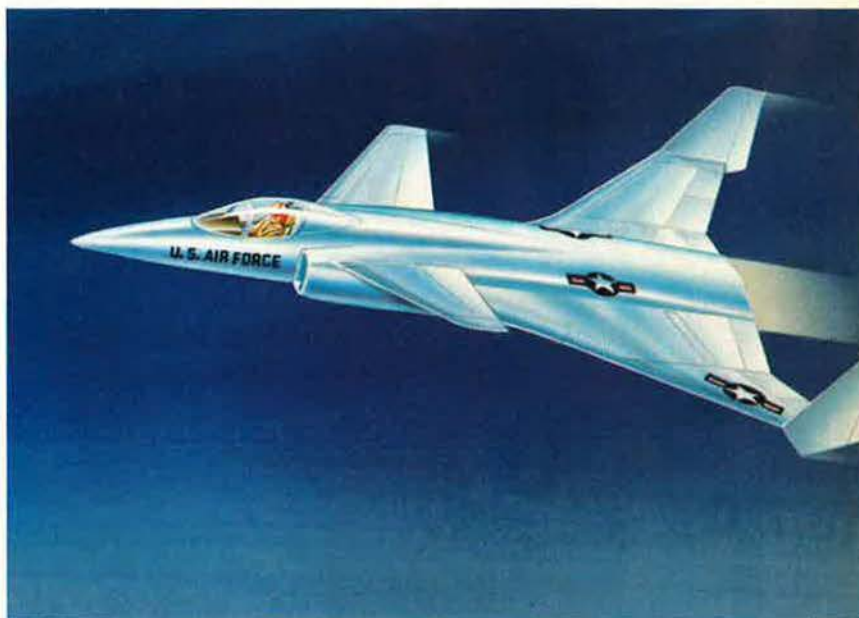
Phase I AFTI studies in 1974 and 1975 involved three major aerospace companies and culminated in three different design proposals. TOP: McDonnell Douglas proposed a vectored-lift fighter (VLF) using a variable-incidence wing (outside of the nacelle), a movable chin canard, and fully movable vertical stabilizers. MIDDLE: Fairchild proposed a 2-D nozzle. BOTTOM: Rockwell stressed canards and composite materials.
