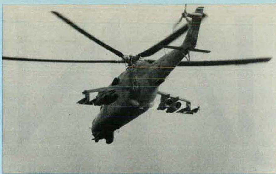
This photograph of the Mi-24 gunship, Hind-D , shows the repositioned tail rotor, now standard on all but early models of this helicopter
