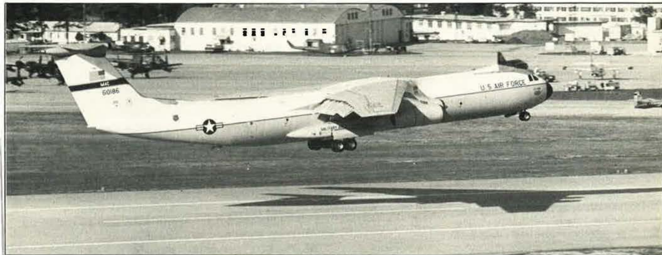
USAF's YC-141B stretched StarLifter takes off from Dobbins AFB, Ga., on its maiden flight. The airlifter has a projected productivity increase of up to forty-five percent—on a fleet basis the equivalent of adding ninety to 120 aircraft to the airlift fleet, officials said.
