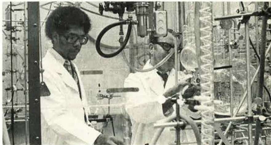
A distillation unit at Aerospace Guidance and Metrology Center, Newark AFS, Ohio, reclaims fluids used in aircraft and missile inertial navigation systems.
