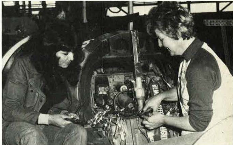
Aircraft electricians at the Ogden Air Logistics Center, Hill AFB, Utah, work on an F-4 Phantom electrical system. AFLC employs some 83,000 civilians.
