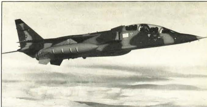
Resplendent in desert camouflage, this Anglo-French-built, two-seat Jaguar International fighter is destined for the Oman Air Force under a multimillion-dollar contract negotiated by the Middle East nation in 1974.
