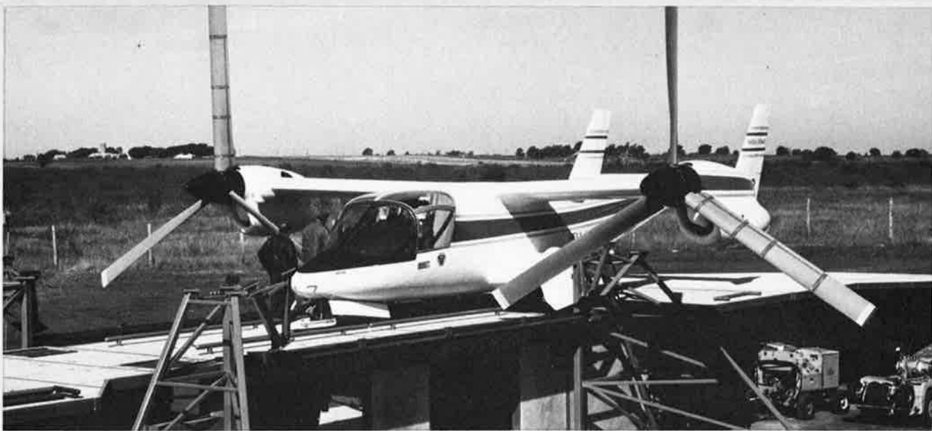
First XV-15 on ground test stand, with propeller/rotors in cruise configuration
