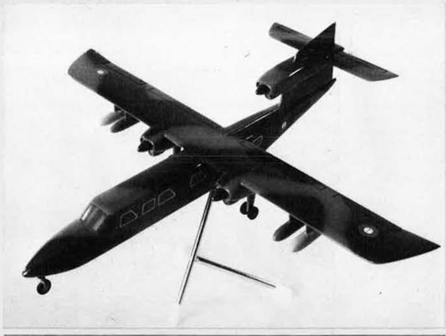
Britten-Norman Military Trislander. This model of the maritime patrol version shows the aircraft with underwing tanks and life raft/survival packs
