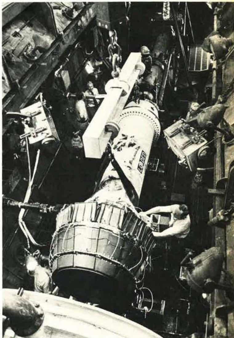
Key feature of MX is the variable-geometry of its upper stage nozzle, shown here in an Arnold Engineering Development Center test cell.
