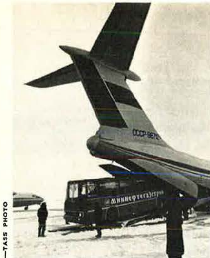
Dished fairing on tailcone of this Il-76 (NATO 'Candid') suggests it was used as testbed for military flight refuelling version or for rear gun turret
