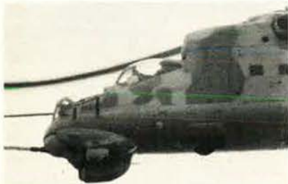
First photo of gunship version of Mil Mi-24 (NATO 'Hind-D'), showing four-barrel Gatling-type machine-gun in turret under nose
