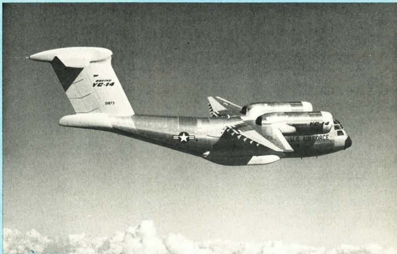
First prototype of the Boeing YC-14 advanced medium STOL transport (two General Electric YF103-GE-100 turbofan engines)
