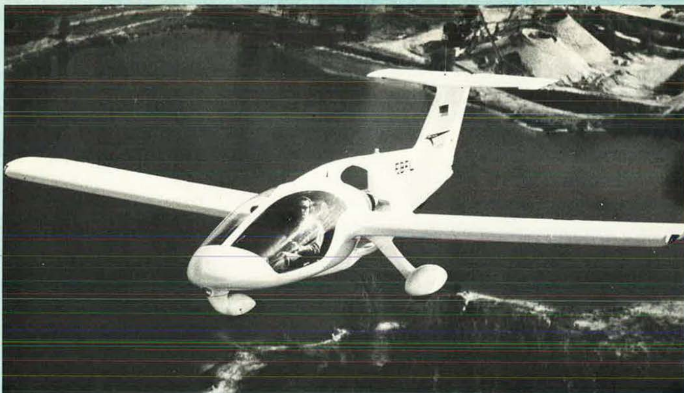
Second prototype of the RFB/Grumman American Fanliner, with integral ducted propeller
