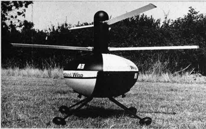
Wisp has a 1.52 m (5 ft) diameter co-axial rotor system and a body 0.61 m (24 in) in diameter and 0.41 m (16 in) in depth
