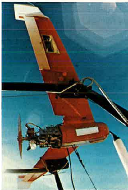
Top view is of Melpar's single-tail-boom pusher powered by Roper 3.5-hp., single-cylinder, two-cycle engine. Above is another Melpar design on its launcher. Northrop's "Flying Wing" mini-RPV, right, is powered by a Kolbo D274 8.5-hp., twin-cylinder, two-cycle engine.
