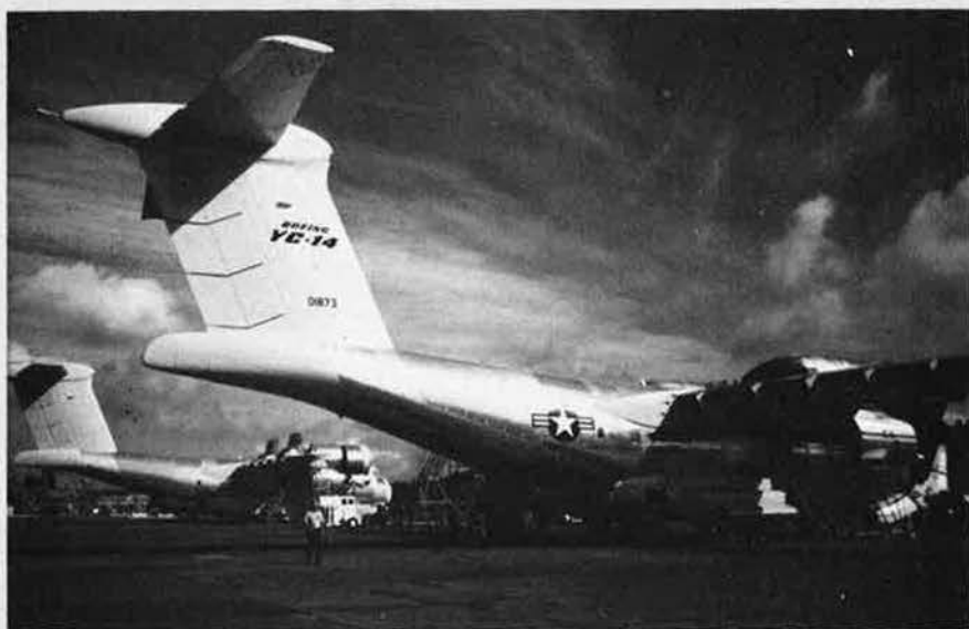
ABOVE: Both prototypes of the YC-14 at Boeing-Seattle. Each aircraft has its rear loading ramp/door partially open. BELOW: Features of the YC-14 shown in this view include large curved flaps, vortex generators in engine exhaust flow, rear loading ramp, and double-hinged tail control surfaces
