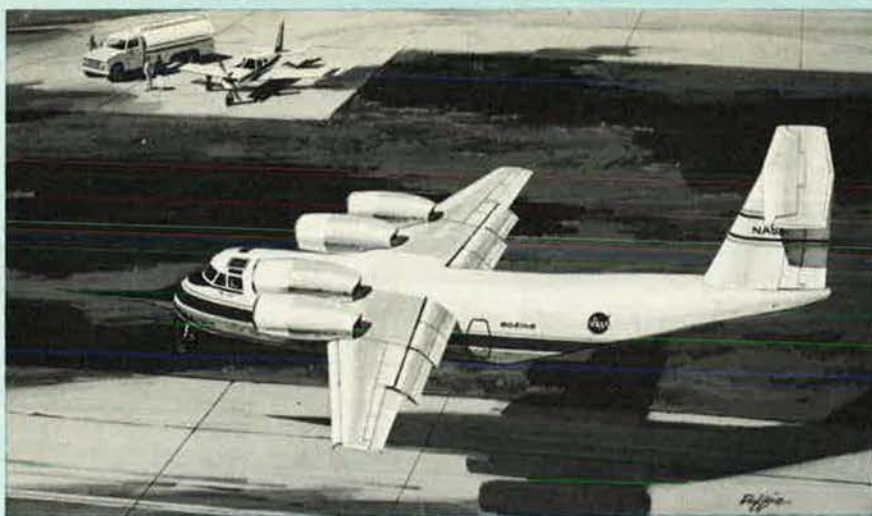
Artist's impression of the C-8A Buffalo which Boeing Commercial Airplane Company is modifying for NASA as a quiet short-haul research aircraft (QSRA). Scheduled to fly in the second half of 1978, the QSRA will be powered by four Avco Lycoming YF102 overwing turboprops and will have a similar wing lift system to that of the YC-14. It will be used to investigate methods of reducing airport congestion and noise
