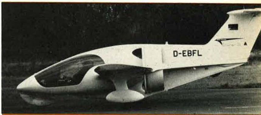
A supercritical wing, with NASA-developed winglets, coupled with Rolls-Royce Spey turbofans, will give the Gulfstream III (above) thirty-five percent more range and seventeen percent higher cruise speed than the Gulfstream II. Right, the Rhein Flugzeugbau Fanliner with cabin design by Luigi Colani, a ducted fan driven by an Audi/NSU Wankel-type rotary engine, and Grumman American wing. Below, Bell's XV-15, built for NASA/US Army testing, represents the end product of a quarter century of tilt-wing development by its manufacturer.
