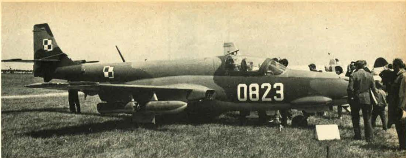
The Polish-built TS-11 Iskra has been in production since 1963. Both two-seat trainers and this single-seat light attack version are being produced.
