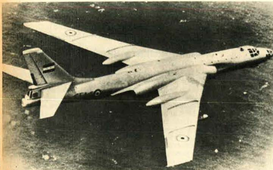
The air forces of Egypt and Iraq are equipped with Soviet-made Tu-16 bombers, with a range of about 4,000 miles and a bomb load of some 20,000 pounds.
