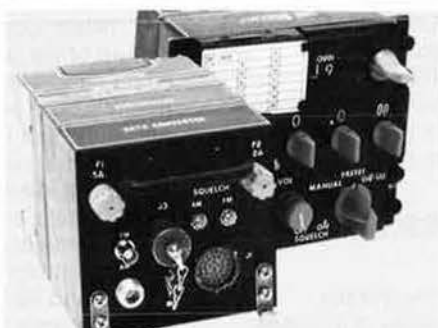
CA-663(R)/ARC-164 VHF-AM/FM remote RT and control
