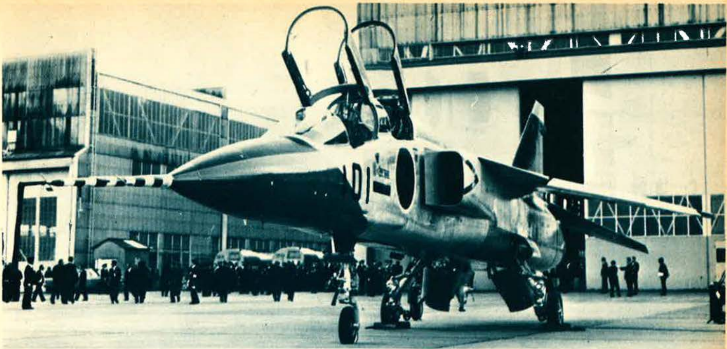
The Japanese Air Force's T-2 jet trainer was the first supersonic aircraft to be developed by the Japanese aircraft industry. It has a Mach 1.6 top speed.
