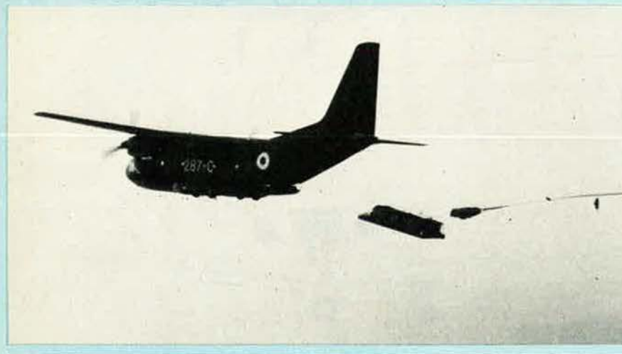
Air delivery of a 5,000 kg palletised load by an Aeritalia G222 twin-turboprop transport
