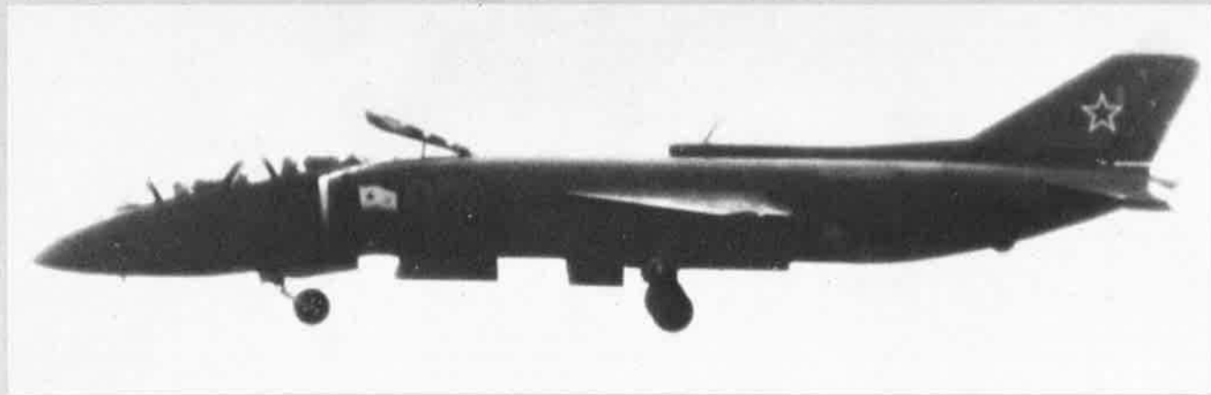
First photograph of the two-seat Forger-B version of the Yak-36. Note the deepened and lengthened nose containing the second cockpit, and the continuous canopy over both cockpits
