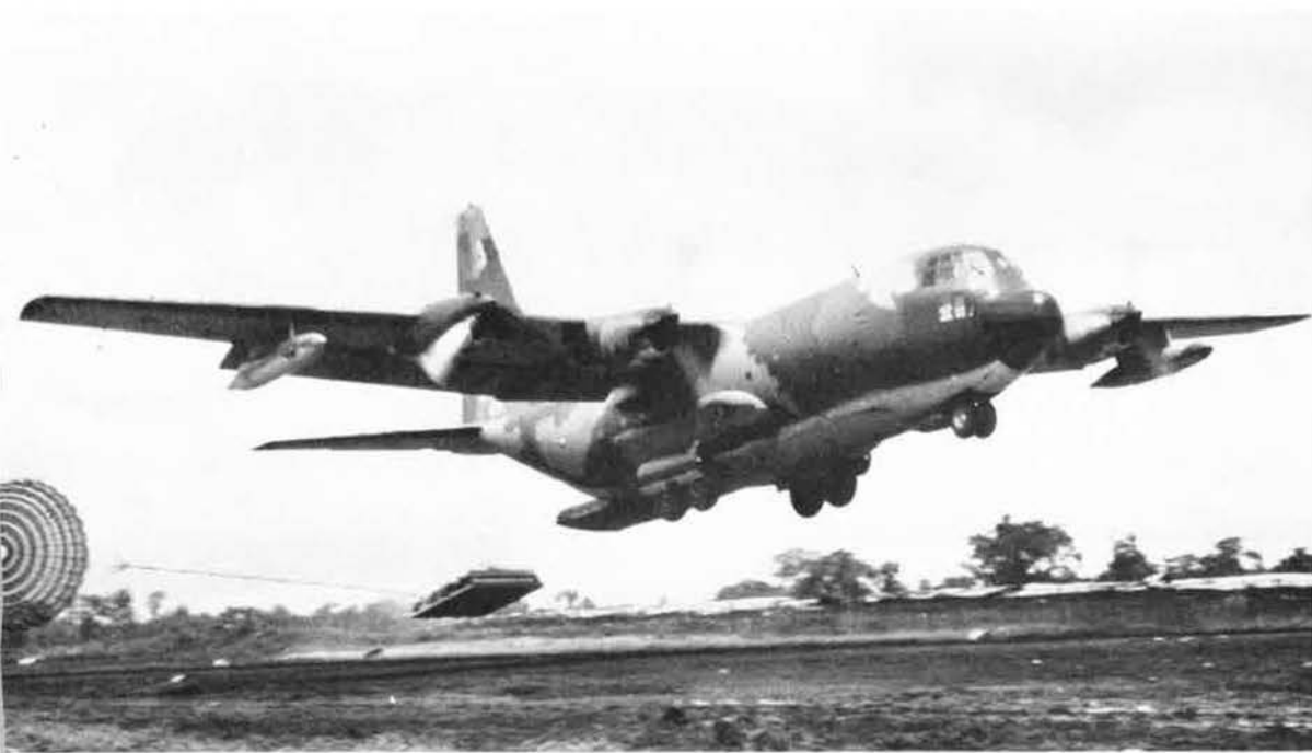
Using the LAPES delivery technique (left) C-130s can deliver equipment as large as the Army's Sherman tank. Below, these USAF Herks are two of more than 1,300 C-130s in use by thirty-seven countries.
