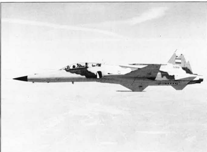
The F-5F fighter/trainer is the two-seat companion to Northrop Corp.'s F-5E single-place tactical air defense fighter. Initial deliveries of the F-5F have begun and orders for the versatile aircraft now exceed ninety worldwide, the company reports.
