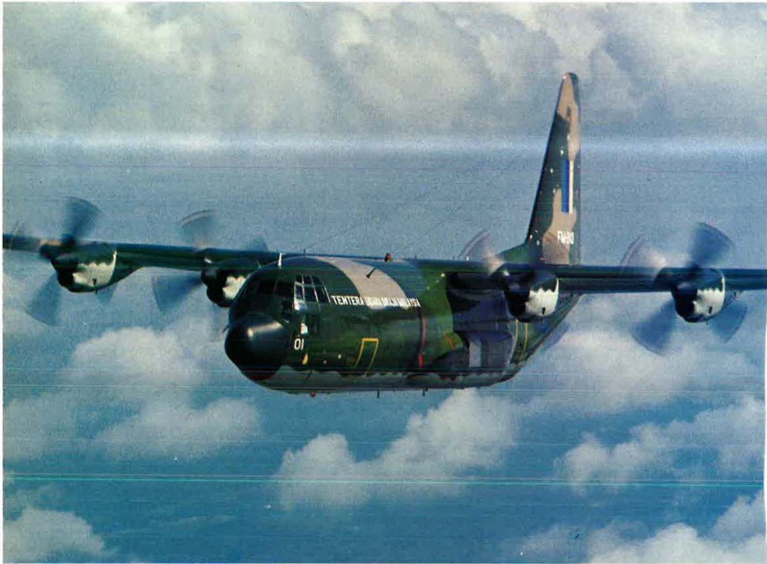
The latest C-130H, represented by the Malaysian Air Force Herk (above), has fifty percent more range than earlier models. Worldwide, C-130s, including USAF versions in battle dress (right), have logged more than 11,000,000 flight hours.
