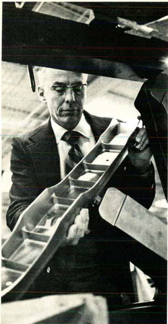
N. E. Klarquist of the Manufacturing Technology Division of the Air Force Materials Laboratory is shown fitting an isothermally forged torque rib into an F-15 horizontal stabilizer.
