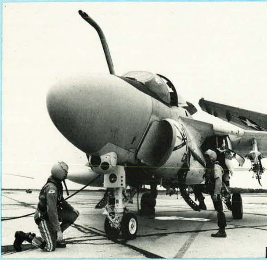
US Navy pilot checks the TRAM turret on an A-6E test aircraft before take-off (Howard Levy)
