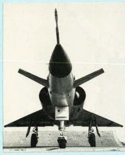
The retractable 'moustache' foreplanes fitted to the Dassault Milan
