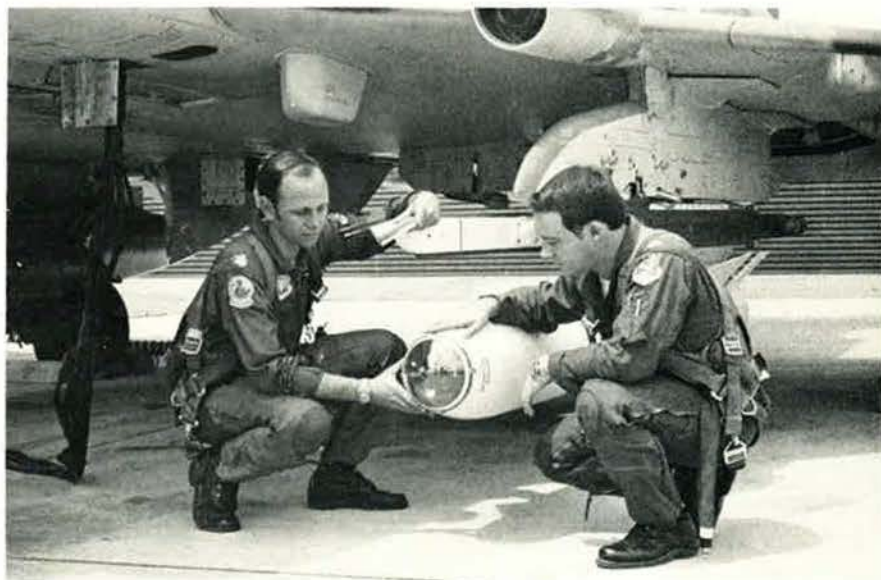
Cpts. Larry Ernst and Charlie Sallee, both assigned to Luke AFB, Ariz., preflight an AGM-65 Maverick prior to launch on a tactics training mission. Each F-4 Fighter Weapons School student fires a Maverick during the terminal-guidance portion of the four-month-long course.
