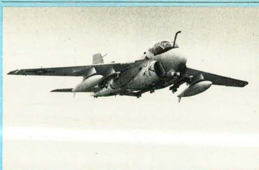
When this photograph of the TRAM-equipped A-6E was taken, the undernose turret was tracking the photographer (Howard Levy)
