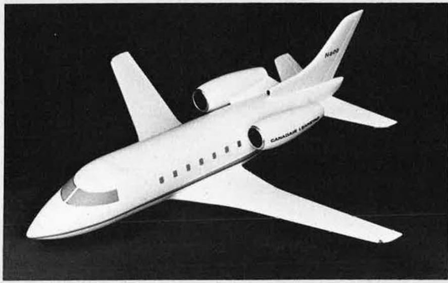
Model of the wide-bodied Canadair LearStar 600 (two Avco Lycoming ALF 502 turbofan engines)
