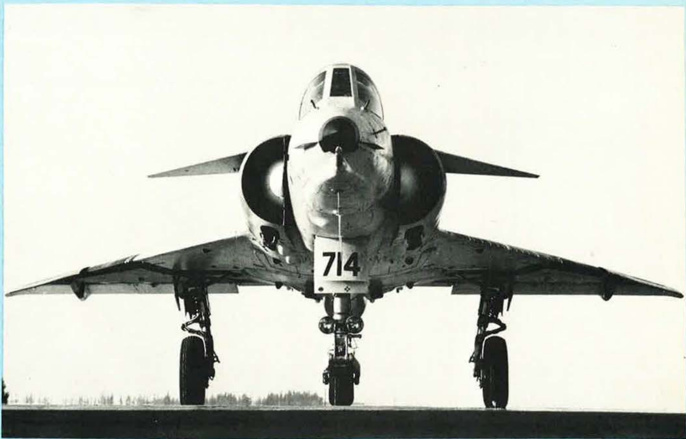
Newly added canards and nose strakes are shown clearly in this ground view of the IAI Kfir-C2
