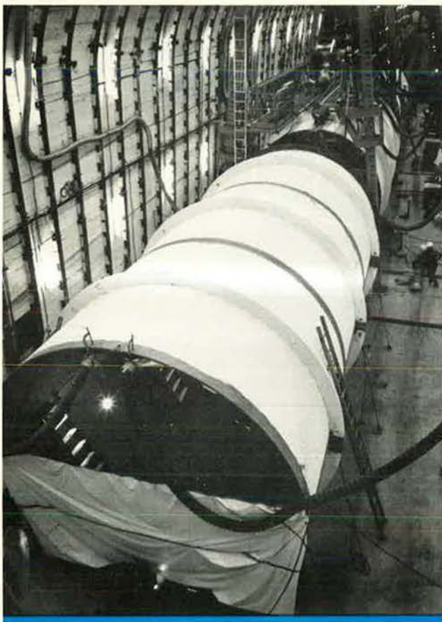
Underground testing at a Nevada site provides information about shock, thermal, and nuclear radiation effects on military hardware. Testing takes place in tunnels drilled into the mountainside.
