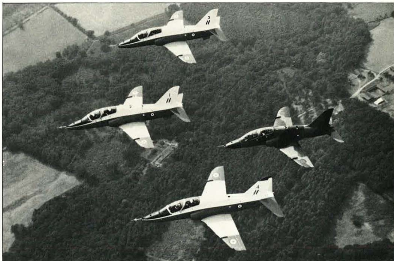
The RAF is expecting first deliveries of the Hawk ground attack/trainer in October. The Hawker Siddeley aircraft is capable of toting 5,000 pounds (2,270 kg) of ordnance on its five pylons. RAF has on order a total of 175 Hawks.
