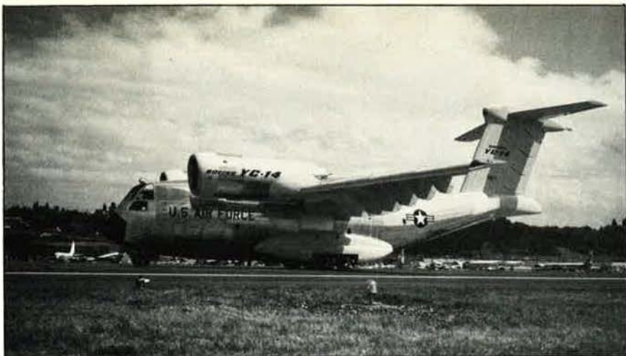
The YC-14—Boeing's contender in the USAF short-field transport program—began taxi tests in July. The plane, powered by two CF6-50 engines, is designed for operation on primitive runways while hauling a wide variety of outsized cargo, including heavy Army ground-combat equipment.
