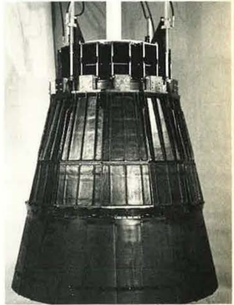
A key element of M-X propulsion efficiency is ENEC, the extendable nozzle exit cone, shown in the above sequence in a stowed position, left, at the mid-rotation point, center, and fully deployed, right. One ENEC advantage is better space utilization.
