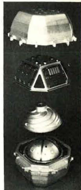
AIRS guidance system weighs 115 pounds. Its core, the "floated ball," is ten inches in diameter.
