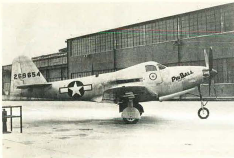
This hand-built RP-63A prototype was followed by more than 100 production models. During the spring and summer of 1945, some 12,000,000 rounds of frangible ammunition were fired by flexible gunners at these target planes.
