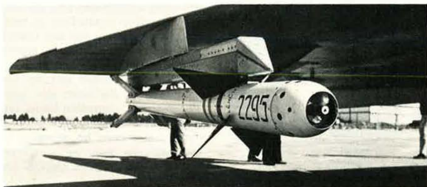
One of the IAF’s most effective weapons in air-to-air combat is this Israeli-built Shafrir missile. The IAF is said to have lost 102 aircraft in the Yom Kippur War, but forty percent of them were to Russian-made SAMs.
