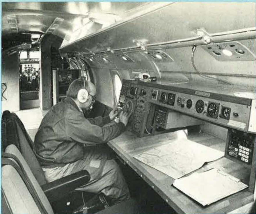
Tactical station inside the main cabin of the Fokker-VFW F27MPA
