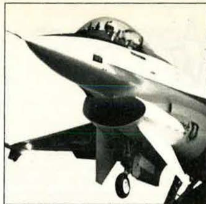
Canards on underfuselage of YF-16 test-bed aircraft improve maneuvering capability. See below.
