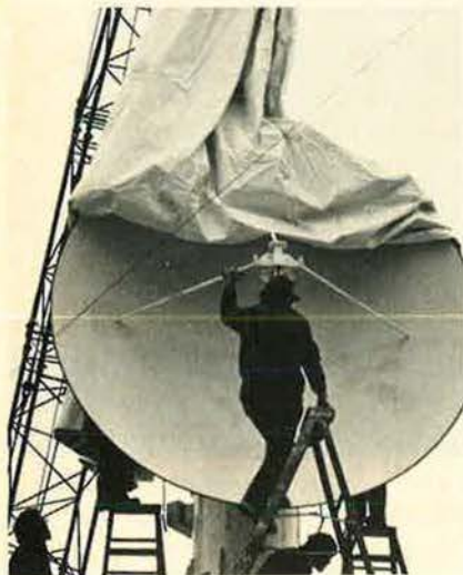
Linked to LES-8 and LES-9 satellites, USAF is testing a new secure, jam-resistant communications system involving a modified C-135 and a special EHF antenna.
