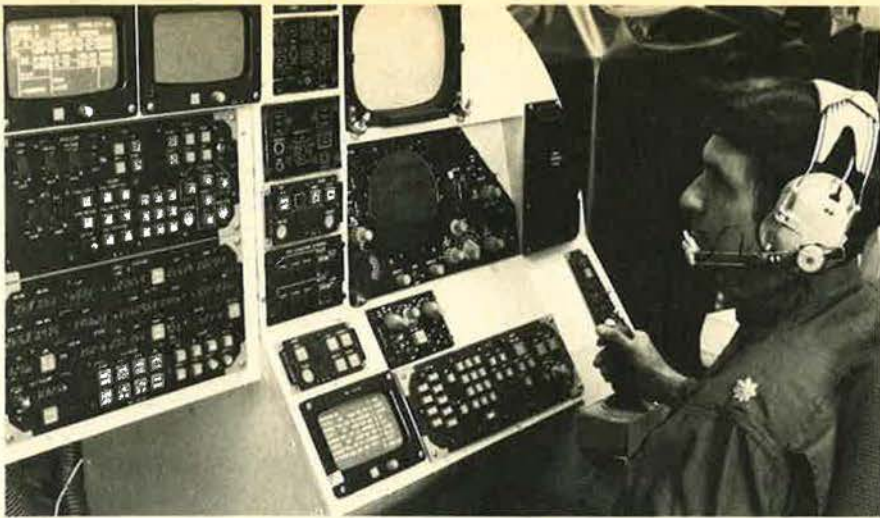
Mockup of B-1's offensive avionics station shows multifunction displays for FLIR as well as alphanumeric data, with round screen below the display for forward-looking radar.
