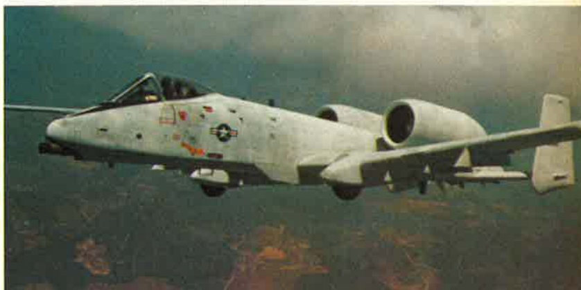
The A-10, the first aircraft designed specifically from the outset for the close-support mission, is scheduled to join the Air Force's operational inventory early in 1978.
