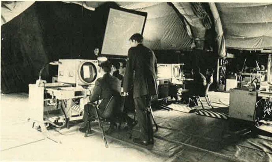
ESD's transportable, computer-controlled display consoles and area viewing screen, enclosed in inflatable shelters, will facilitate tactical aircraft control.
