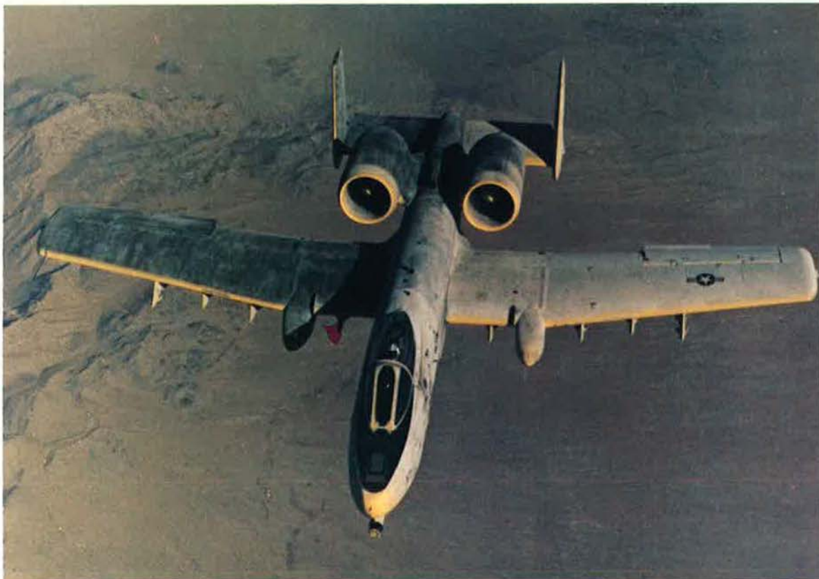
An A-10 undergoes icing tests, with water sprayed from a KC-135 directly in the test plane's path. Note yellowish ice build-up on the leading edges of wings, tail surfaces, the nose, and engine cowlings.
