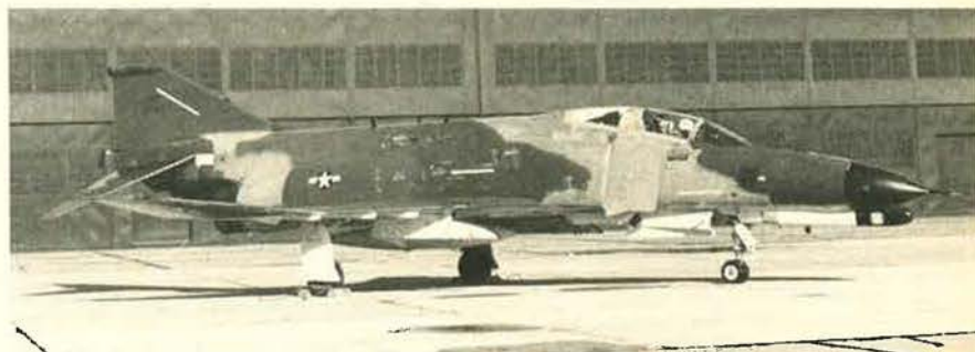
F-4G Wild Weasel, shown here at McDonnell Douglas facility, is currently in flight test. Pod under the nose and pod on the top of tail are added to standard F-4E.
