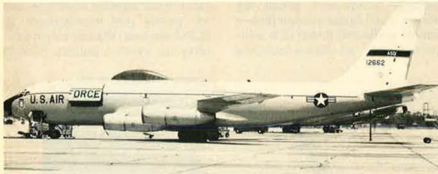
Linked to LES-8 and LES-9 satellites, USAF is testing a new secure, jam-resistant communications system involving a modified C-135 and a special EHF antenna.
