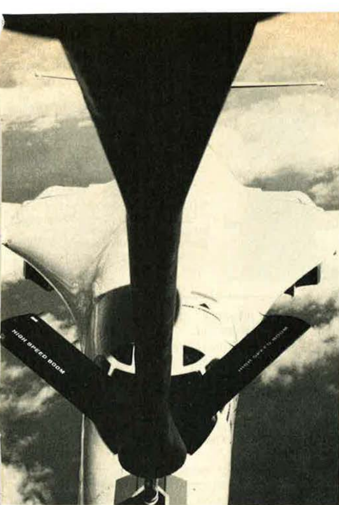
During aerial refueling, the B-1's flight control and thrust responses are rapid. Having the refueling receptacle in front of the pilots provides a good secondary closure rate reference.
