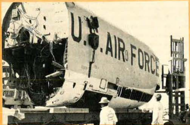
AFLC's Military Aircraft Storage and Disposition Center reclaims B-52 nose section for use in flight simulators.
