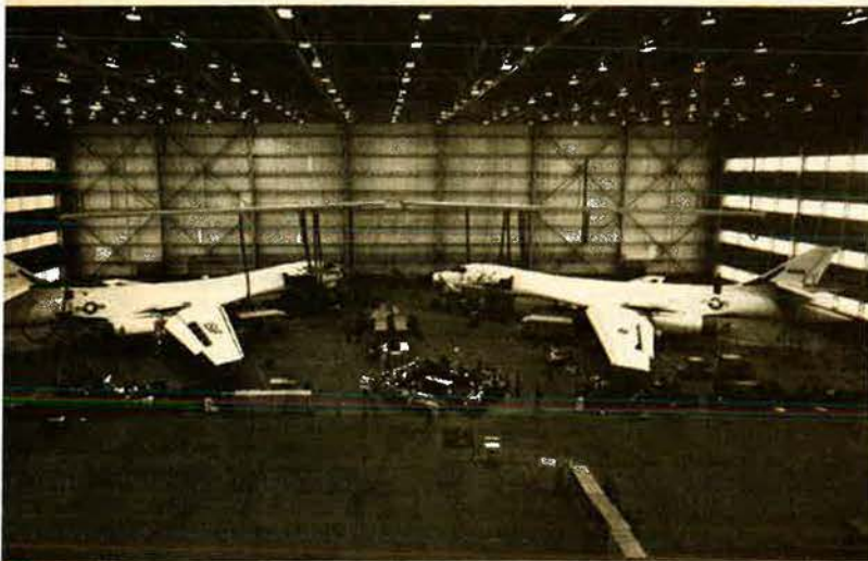
The B-1 is designed to be completely self-sufficient, with onboard APUs providing the necessary power for the ground crew to check out all systems with the built-in Central Integrated Test System computer.
