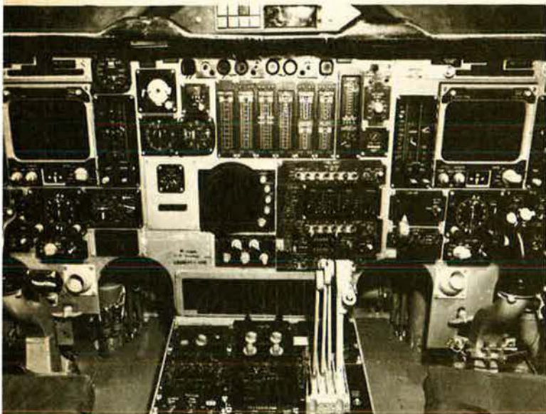
The B-1 cockpit (above) combines optimum instrument layout and exceptional visibility. Unique for an aircraft of this size is the use of a control stick instead of a wheel. The B-1's variable-geometry wing, fully swept in the photo at right, increases efficiency at high subsonic and supersonic speeds.
