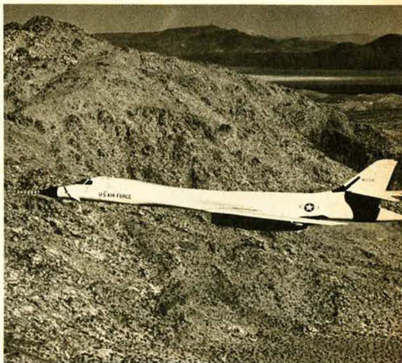
In a high-speed, low-altitude penetration, the B-1 will use terrain masking to avoid radar detection. Its Structural Mode Control System moderates low-altitude turbulence.
