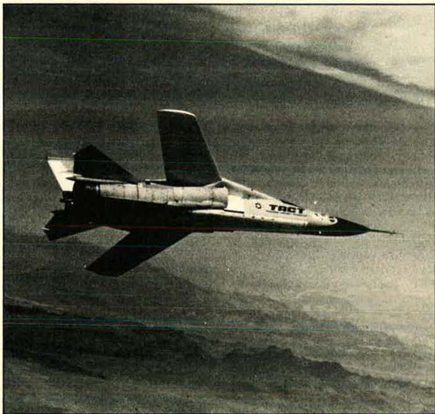
TACT, the joint USAF/NASA Transonic Aircraft Technology Program involving an F-111 with supercritical wings, scored significant gains in the transonic flight regime, including reduced turn radii.
