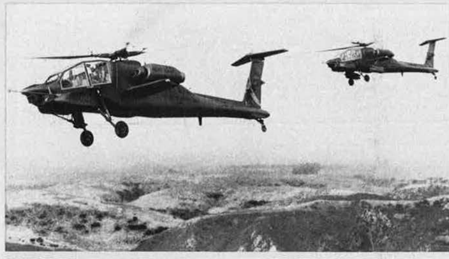
Both Hughes YAH-64 flight test prototype aircraft shown, 22 November 1975, during maiden flight of the aircraft on the left. Note TOW missile pods on aircraft at right
