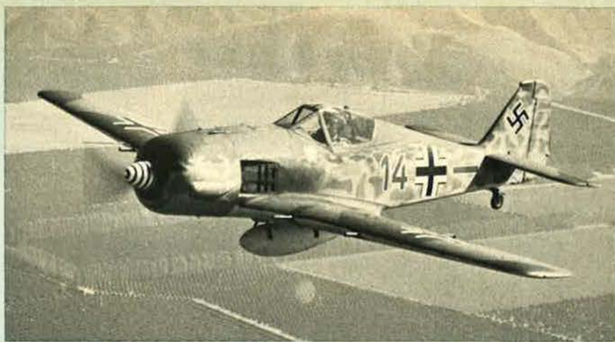
War Aircraft Replicas Focke-Wulf 190, a half-scale reproduction of the wartime German fighter, with a 70 hp Volkswagen engine (Howard Levy)
