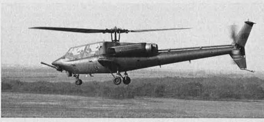
First prototype of the Bell YAH-63 (two 1,536 shp General Electric T700-GE-700 turboshaft engines)
