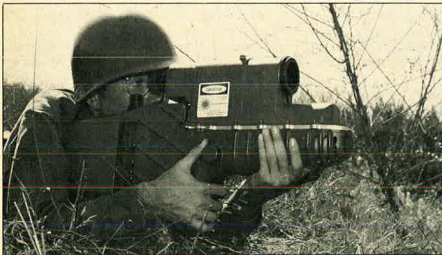
Weighing only thirteen pounds, this lightweight laser designator can be aimed like a rifle to pinpoint targets for laser-homing weapons. Built by Hughes Aircraft Co., the LWLD will first undergo stress testing by the Army Electronics Command, followed by fully operational field tests.
