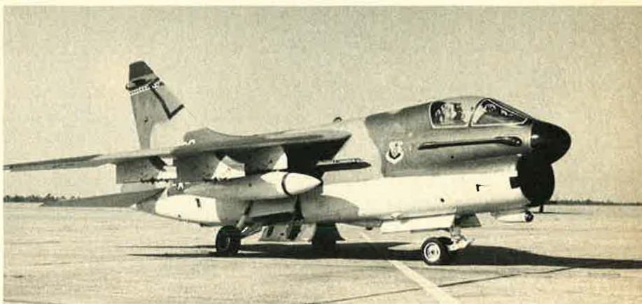
Top: The F-4G Wild Weasel electronic warfare system can be quickly modified in terms of computer software to meet changing threat situations. Bottom: Pave Penny, shown here on an A-7, is a new miniaturized laser search and track system that picks up FAC-designated targets.
