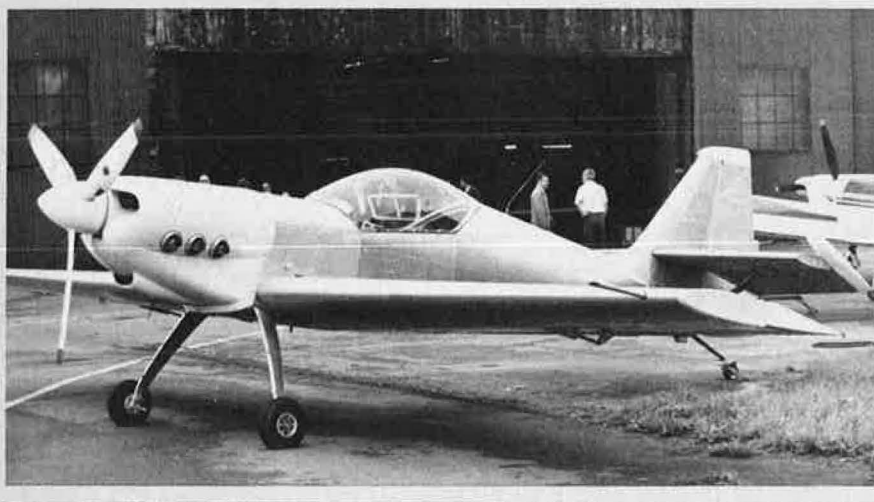
Prototype of the Zlin Z 50 L (260 hp Lycoming AEIO-540-D4B5 engine)
