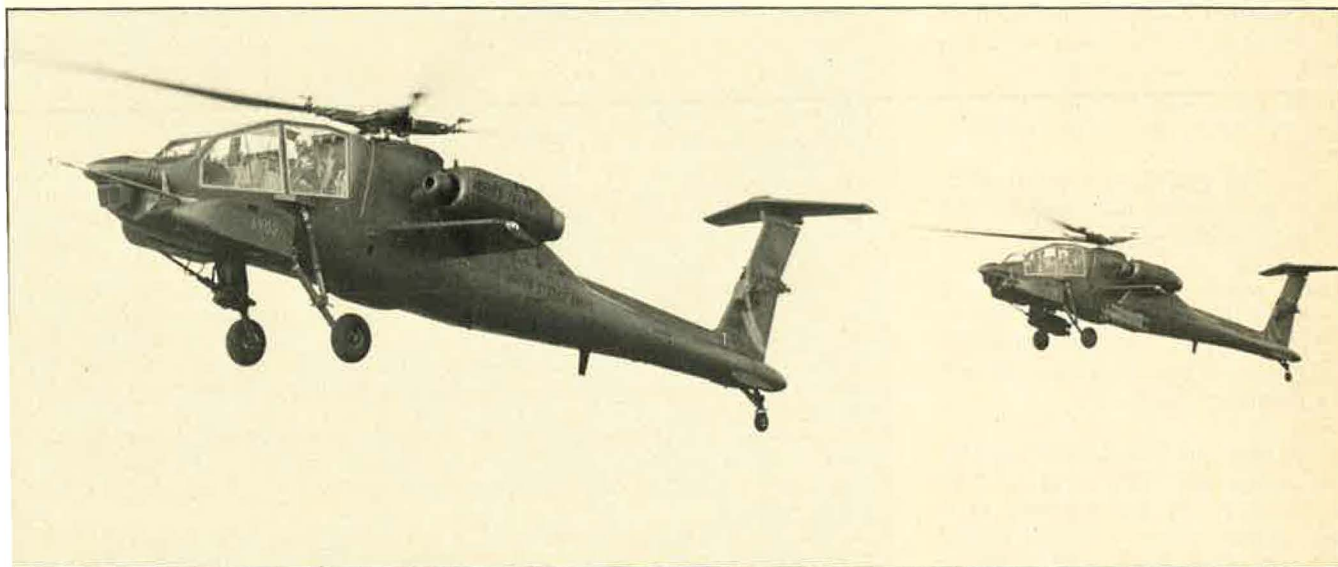
'Insect-like competitors in US Army's Advanced Attack Helicopter program are these two prototype YAH-64s, built by Hughes. They'll be evaluated against Bell Aircraft Co. contenders, with the winner entering the inventory in the 1980s.
