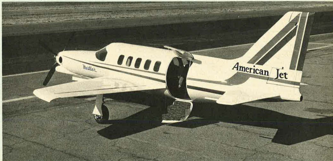
Full-scale mockup of the Hustler, which is expected to be the world's fastest turboprop light aircraft
