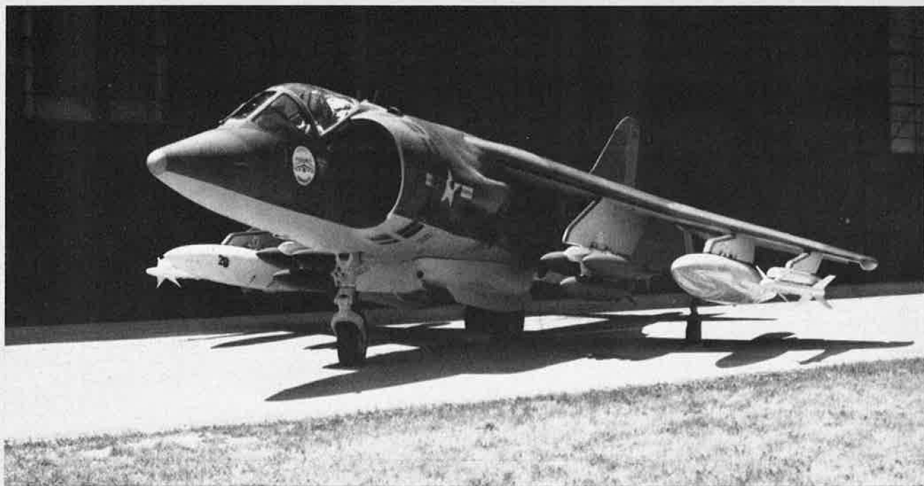
Engineering model of McDonnell Douglas AV-8B Advanced Harrier
