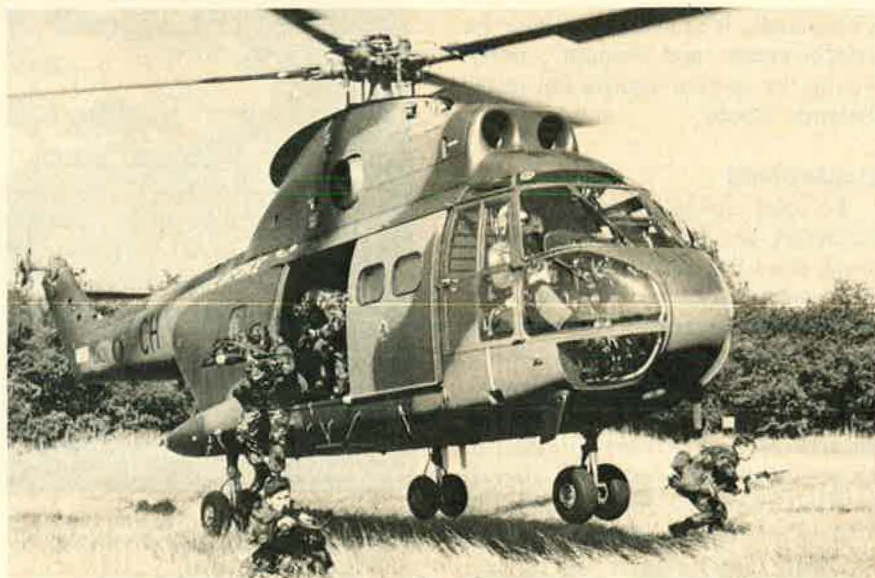
RAF Regiment troops deploy from a Puma helicopter during training exercise. The Westland/Aérospatiale Puma assault helicopter can carry up to sixteen troops or six litters.
