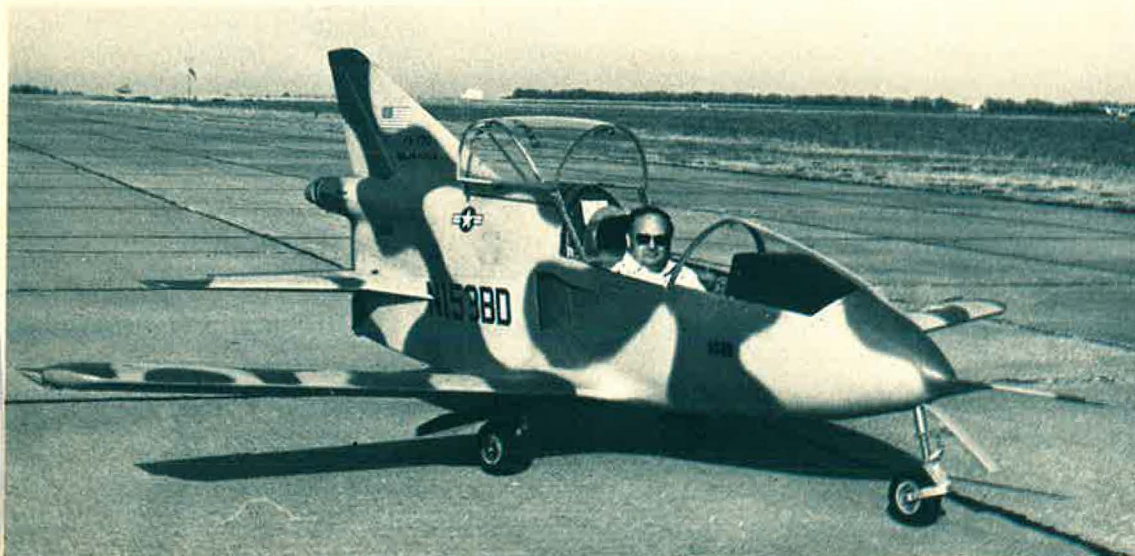
Jim Bede in his 240-knot BD-5J baby jet. The Microturbo TRS 18 turbojet engine develops 202 pounds of thrust. USAF has evaluated it for a variety of possible missions.
