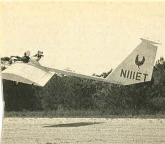
Homebuilts are growing in popularity. This Birdman TL-1, weighing 100 pounds with its 15-hp engine, went on the market in 1975.
