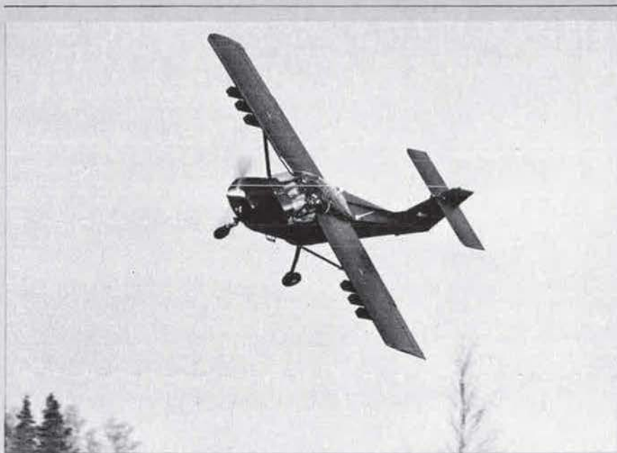
Saab Supporter light multi-purpose military aircraft, with six Bofors Bantam anti-tank guided missiles in underwing containers
