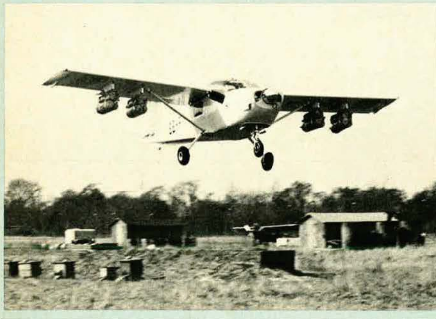
One of the Saab Safaris used for famine relief in Ethiopia, with droppable underwing load
