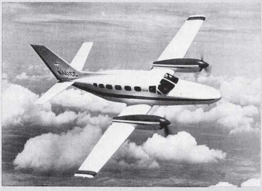
Cessna Model 441 eight/ten-seat pressurised executive transport (two 620 shp Garrett-AiResearch TPE 331-8-401 turboprop engines)
