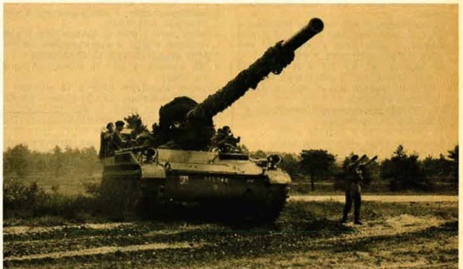
British Army forces deployed to Germany with the British Army of the Rhine include in their equipment these 175-mm self-propelled guns.
