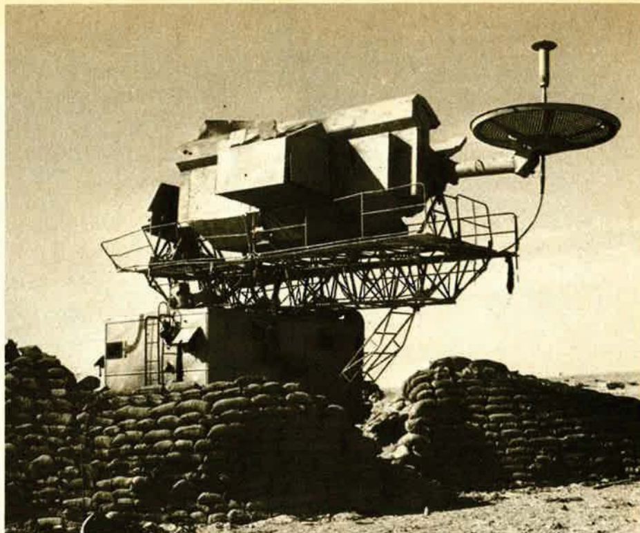
Fan Song radars, part of the SA-2 Guideline surface-to-air missile system, have been supplied by the USSR to defense forces of Egypt, Iraq, and Syria.
