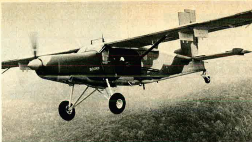
Above, the first of twenty Fairchild AU-23A Peacemakers, military version of the STOL Porter, purchased by the Royal Thai AF. It can be armed with side-firing 20-mm cannon or 7.62-mm Miniguns, and quickly converted to a light transport role. Also new (left) is Bell Helicopter's YAH-63 Advanced Attack Helicopter (AAH), shown after liftoff for its first flight, October 1, near Fort Worth, Tex.
