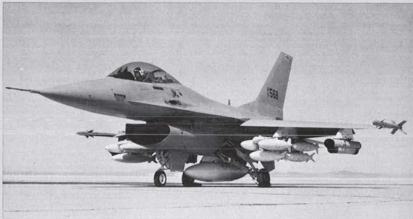
General Dynamics YF-16 single-seat air combat fighter, with typical external load of bombs, Sidewinder missiles, and ECM pods
