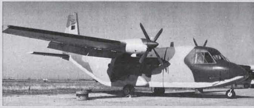
CASA C.212 Aviocar military transport and general-purpose aircraft in the insignia of the Portuguese Air Force
