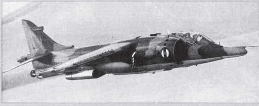
Hawker Siddeley Harrier development aircraft with laser ranging equipment in its nose
