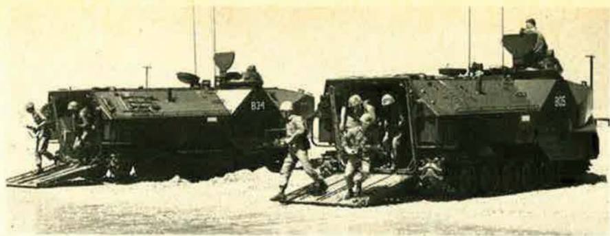
Marines at the double disembark from an amphibious vehicle specifically designed for their mission—the LVTP-7 Amtrack.
