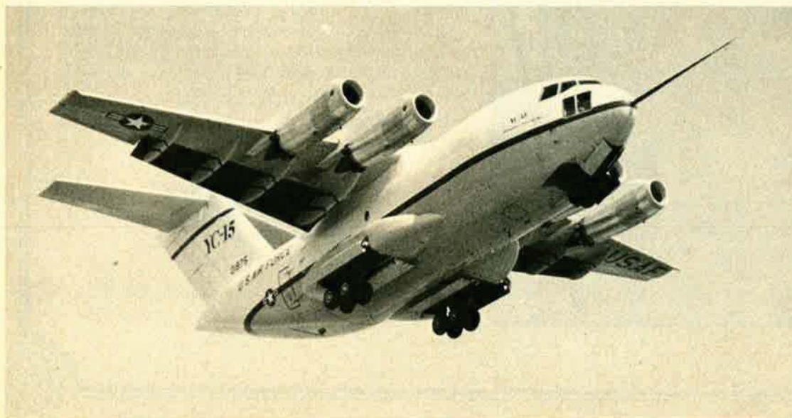
Off on a successful maiden flight is the first entry in USAF's competition to produce an Advanced Medium Short Takeoff and Landing Transport, or AMST (see above). The wide-bodied YC-15, built by Douglas Aircraft Co., is unique for its use of an externally blown flap system and critical-wing design.
