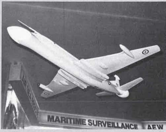
Model of the projected AEW version of the Hawker Siddeley Nimrod (Brian M. Service)
