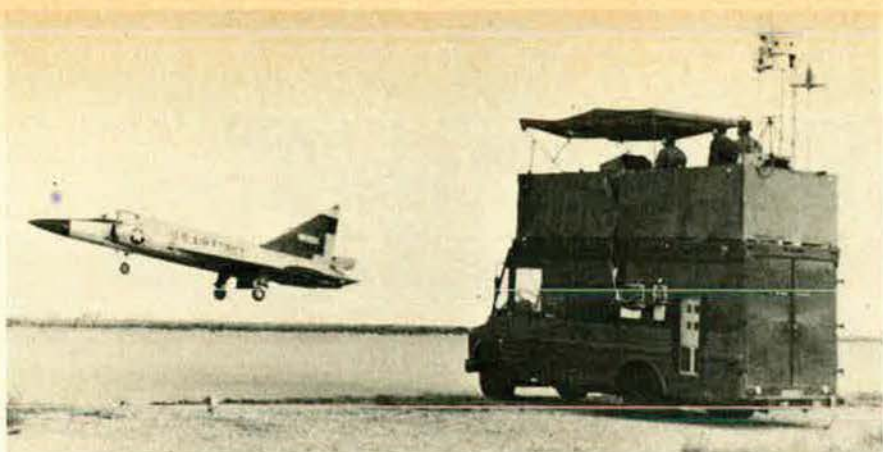
A PQM-102, the first full-size, supersonic drone, takes off unmanned on a recent test flight. USAF plans to convert 127 F-102s to drones. See below.
