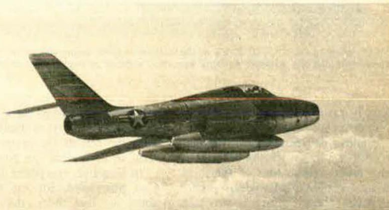
F-84F with two 450s. This configuration, because of the reduced drag, would go as far as the four-tank setup and cruising speed was a respectable Mach .80. The flights to Africa and the return flights to Bergstrom all carried two 450s.
