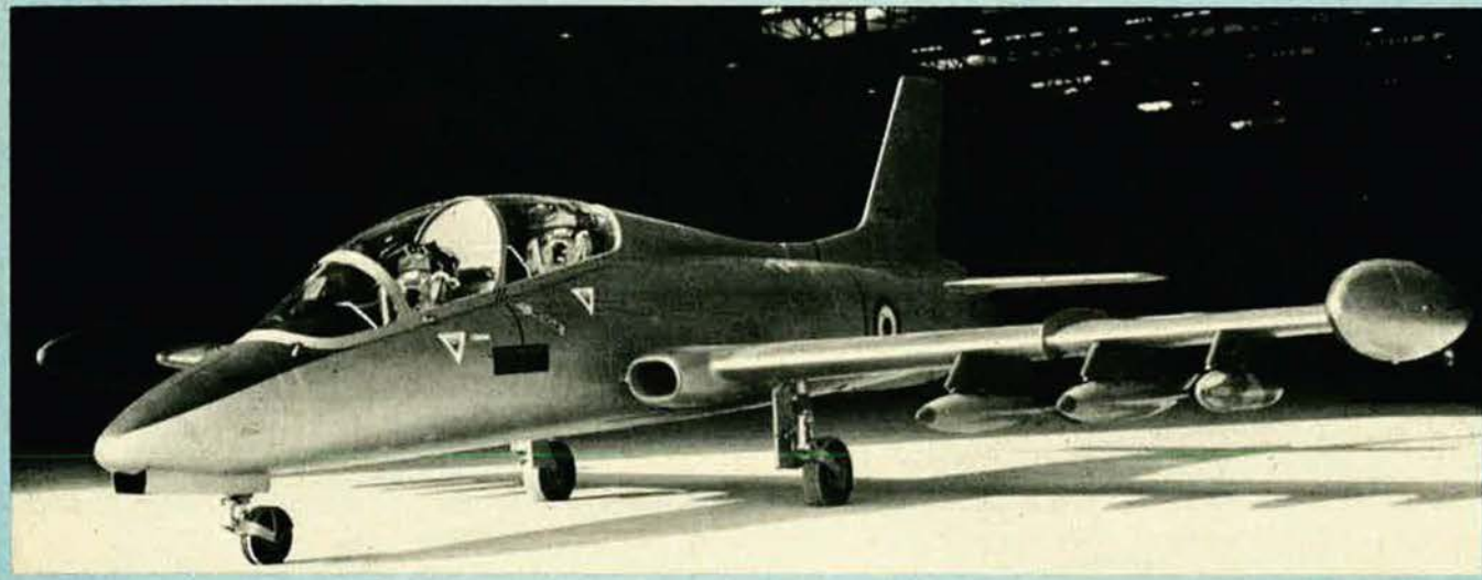
Full-scale mockup of the Aermacchi M.B. 339, showing the raised rear cockpit and underwing armament
