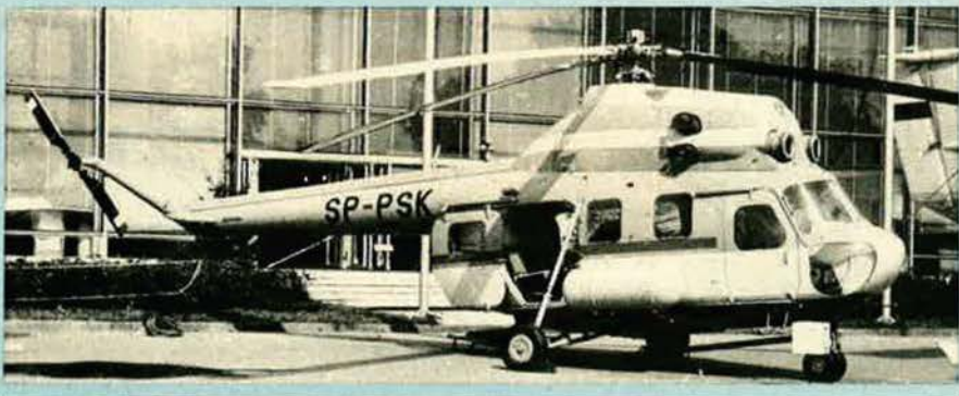
WSK-Swidnik Mi-2M, an enlarged and more powerful version of the licence-built Mil Mi-2
