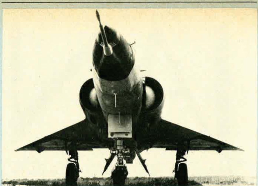
Israel Aircraft Industries Kfir (Lion Cub) aircraft for air defence and ground attack (General Electric J79-GE-17 afterburning turbojet engine)
