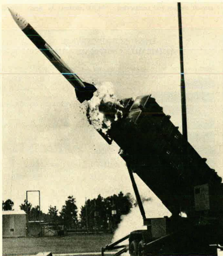
Top, the Boeing Vertol YUH-61A is competing with a Sikorsky developmental helicopter to become the Army's Utility Tactical Transport Aircraft System (UTTAS). Left, a SAM-D surface-to-air missile leaves its canister in a test firing. It is to replace the Nike-Hercules and the Improved Hawk in battlefield defense.
