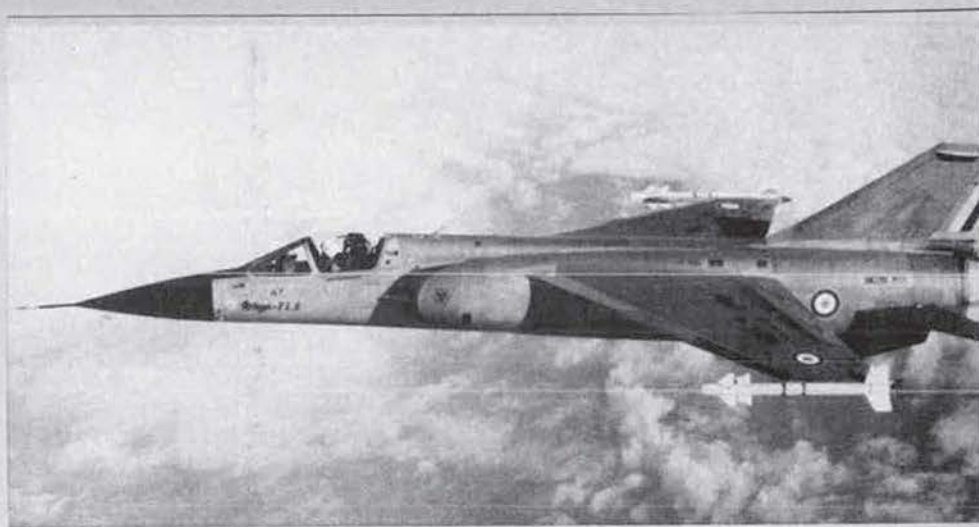
Prototype Dassault Mirage F1-E multi-mission fighter (SNECMA M53 turbofan engine)
