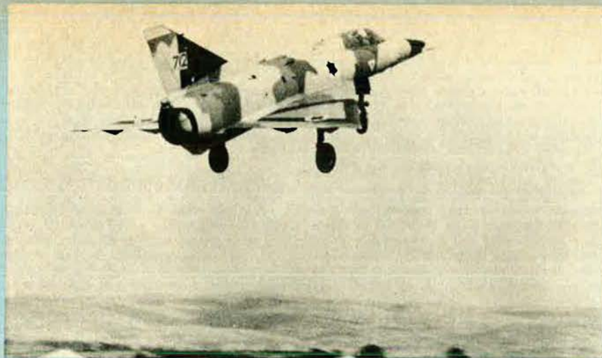
Above, the Kfir taking off. At right, underview of the Kfir in flight shows resemblances to the Mirage III/5. This single-seat, Mach 2.2 plus combat aircraft is developed and manufactured by Israel Aircraft Industries
