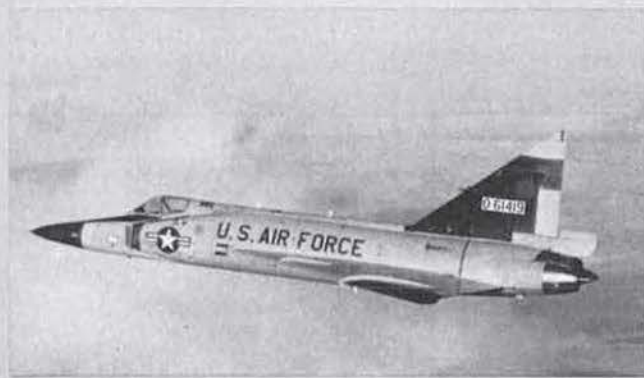
Sperry (Convair/General Dynamics) PQM-102, the first-ever fighter aircraft converted for drone duties with no provision for manned flight
