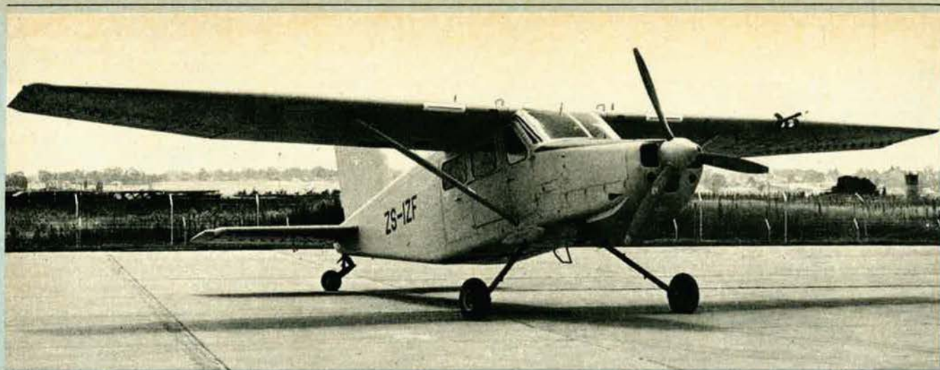
First prototype of the Atlas C4M (340 hp Lycoming GSO-480-B1B3 engine)
