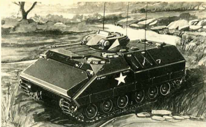
An artist's conception shows another top R&D priority, the Mechanized Infantry Combat Vehicle (MICV). The squad-carrying armored vehicle will have a chain gun or a Gatling gun as well as firing ports for infantrymen inside.
