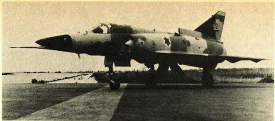
Israeli-built new Kfir fighter-bomber looks like France's Mirage V and has US J79 engines.
