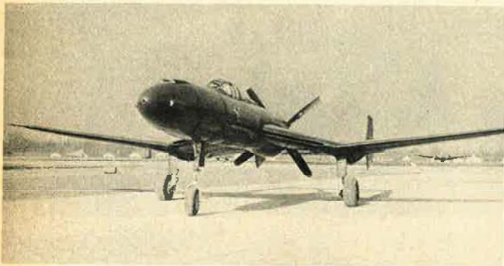
Engineering changes more than doubled the XP-54's design weight, and the resultant speed loss doomed the aircraft.
