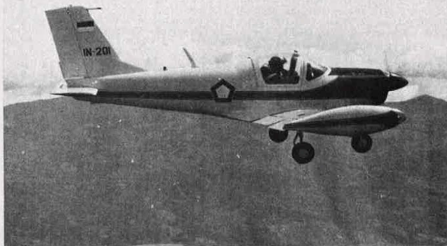
First prototype of the Lipnur LT-200 light aircraft, based on the American Pazmany PL-2
