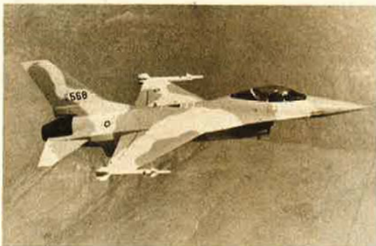
Initial operational testing of the F-16 will involve two prototype aircraft. Phase II will begin with delivery of the first of twelve preproduction aircraft.
