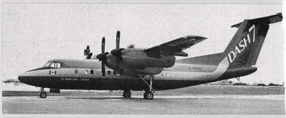
De Havilland Canada DHC-7 Dash 7 "Quiet STOL" transport (four 1,174 ehp UACL PT6A-50 turboprop engines)
