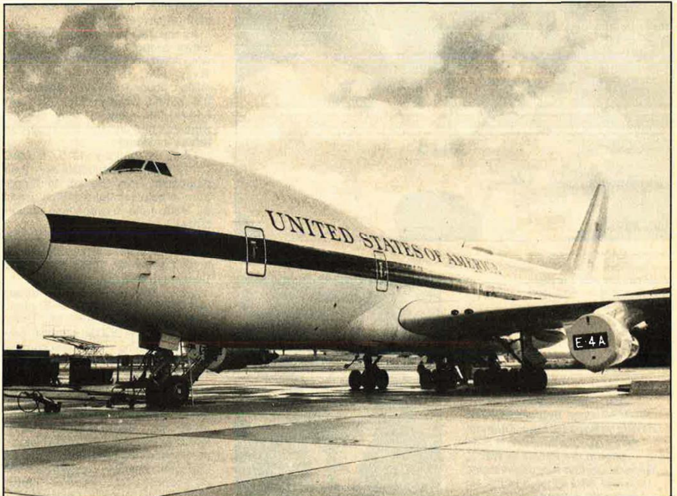
The first E-4A, equipped with command control and communications gear to operate as a National Emergency Airborne Command Post, is at Andrews AFB, Md.
