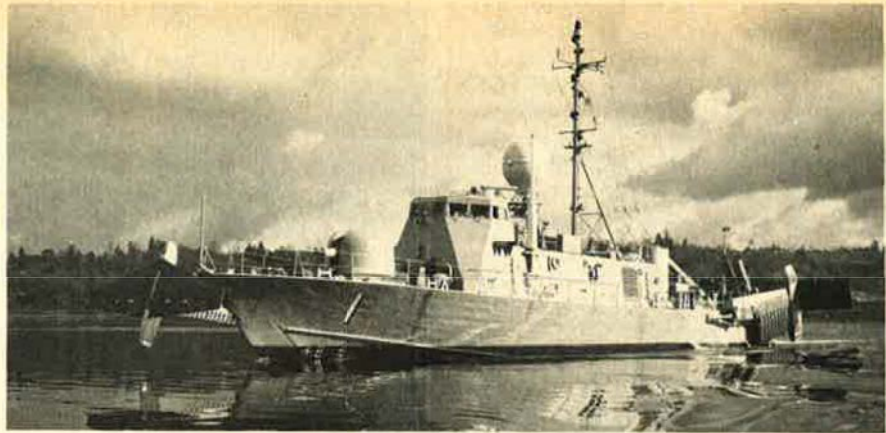
Under way for the first time, the Navy's new Patrol Hydrofoil Missile Ship Pegasus is the subject of a hullborne trial on Seattle's Lake Washington. The ship, built by a Boeing division, can hit better than forty knots.
