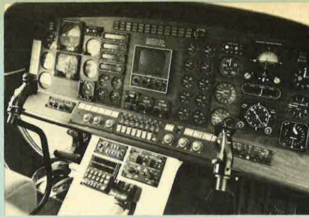
Full IFR instrument panel, complete with digital readout area navigation and communications system, installed in S-76 mockup
