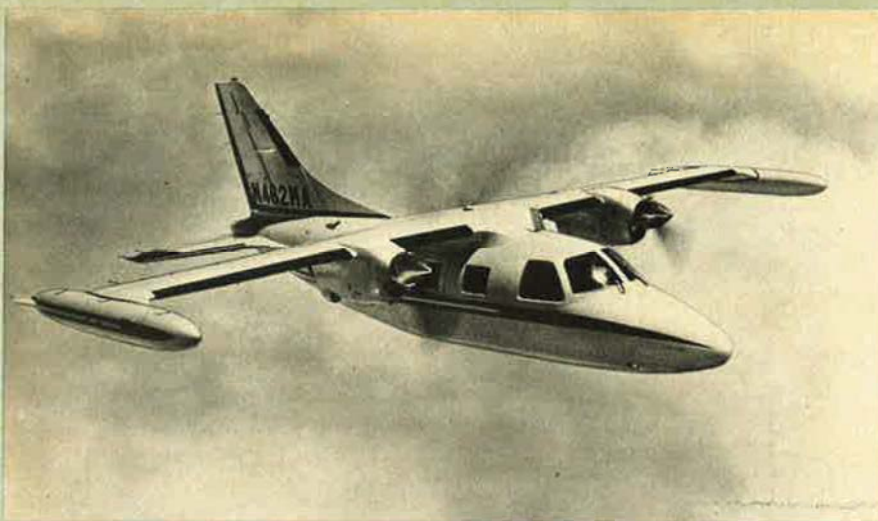
Mitsubishi MU-2M seven/nine-seat business aircraft (two 724 ehp Garrett AiResearch TPE 331-6-251M turboprop engines)
