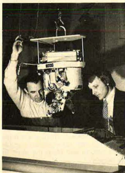
Forward-looking infrared viewing device for the B-1 is undergoing tests at Boeing's Wichita Division. Built by Hughes, it will provide terrain image in any weather, day or night.
