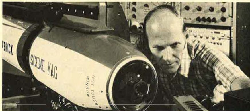
Unique sight allows this new AGM-65B Scene Magnification Maverick missile to spot, lock on to, and be launched against a target at longer range than the standard Maverick, produced since 1972 for USAF by Hughes Aircraft Co.
