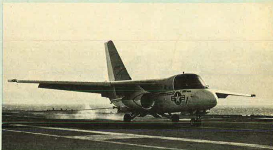
Lockheed S-3A Viking anti-submarine aircraft undergoing carrier suitability tests on the USS Forresteral (US Navy)
