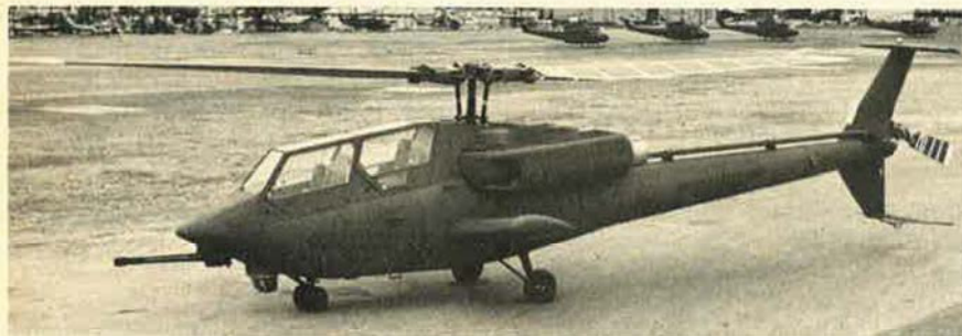
Bell's YAH-63, ground test vehicle for Army's new Advanced Attack Helicopter, under development.
