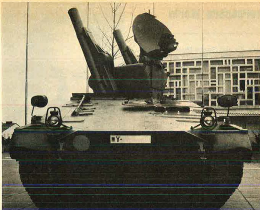
The Roland is a Franco-German-designed all-weather, short-range, vehicle-mounted SAM that US Army plans to buy in large quantities over the next decade. The weapon is to be built in the US under license (see adjacent item).
