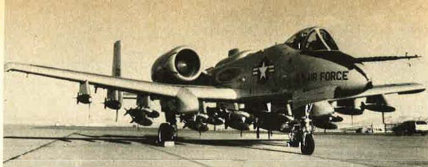
Undergoing certification flight tests, the Fairchild Republic A-10 close-support aircraft recently hit its stride with a maximum load of twenty-eight bombs and a takeoff weight of 45,521 pounds. During flight, the plane withstood four Gs.
